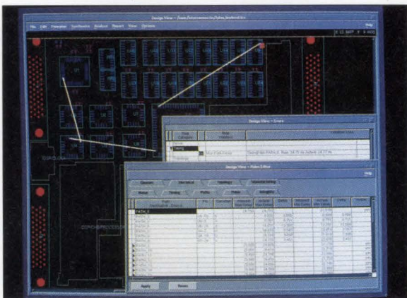
The IS timing-driven floor planner computes slack allocation in real time for all critical timing paths. It displays violations graphically and in tabular form.
