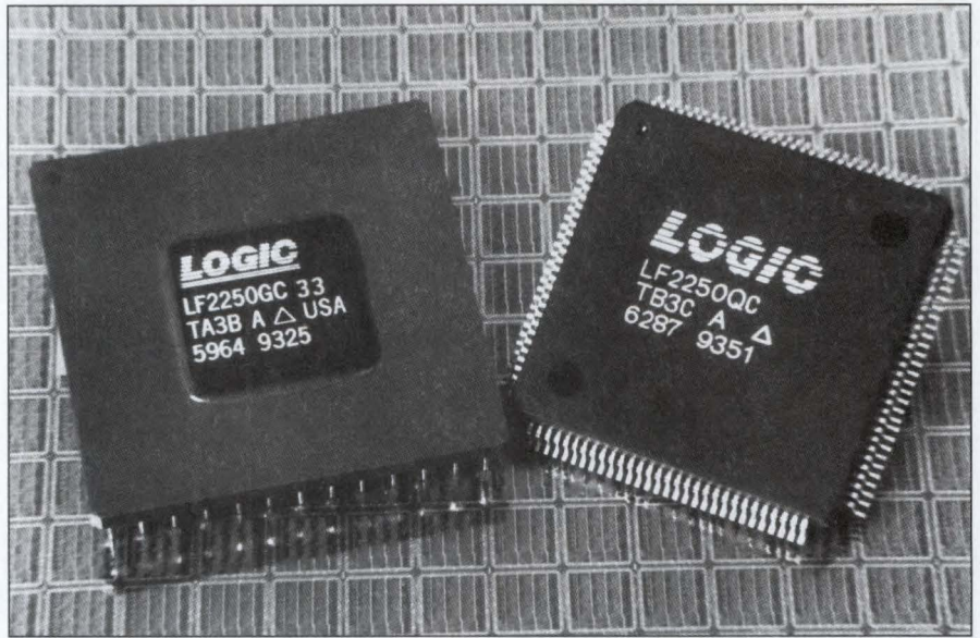
Packages exhibit vastly different electrical characteristics, so choose carefully. The pin-grid array, for instance, has wide pin-to-pin variations in on-chip delays. The QFP has more consistent lead lengths, but has a greater lead inductance. (Photo courtesy Logic Devices)
