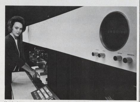
Handwritten numbers can now be read directly into a computer by means of IBM's 1287 optical reader. Designed for use with the company's System/360, the machine can recognize numbers and five different hand-printed alphabetic characters pencil-written on a variety of business documents.
