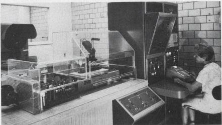
Automatic traveling-wave tube inspection system checks for production errors. Developed by RCA the device measures the pitch of helixes.
