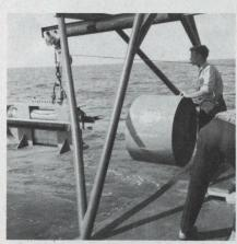
Westinghouse version of SLS fish is prepared for launch. Main frame of the unit is 6-in. steel I-beam. Transducer cases (black stripe) are along the beam sides, the electronic package is above, the batteries are below.
