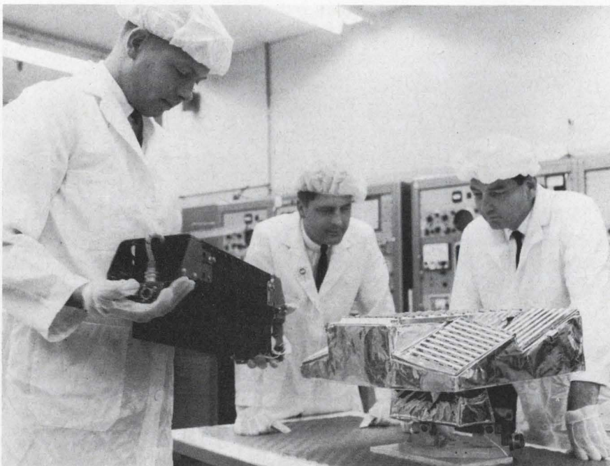
Electronics portion of LEM landing radar system together with aluminum-coated planar array antenna weighs 32.7 pounds.
