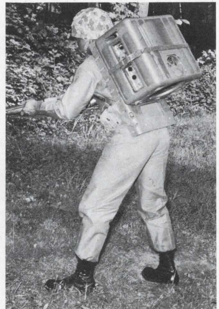
Portable thermoelectric generator weighs 35 pounds, with fuel.
