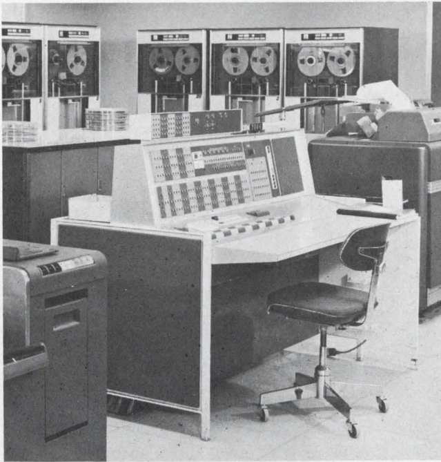
NET-1 may be run on several computers, IBM 7040/44, 7090/94 (as shown) and 360/65 with 7094 emulator.
