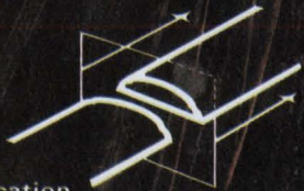
Illustration is 1400X magnification cross-section through selectively plated contact at point shown
