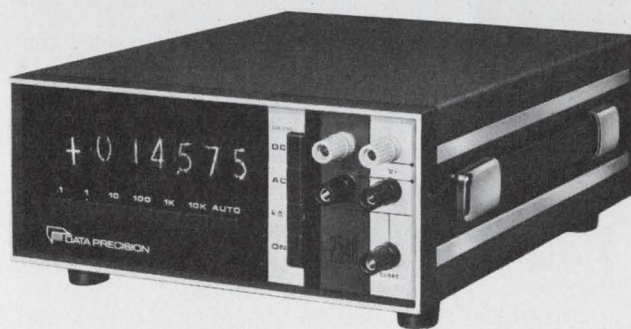
Model 2540, 5½ digits. DC volts, AC volts, Resistance, Voltage Ratio. Auto-ranging. Auto-Polarity. Isolated BCD outputs. Remote triggering. Remote ranging. Basic accuracy ±0.001% f.s. ±0.007% rdg ±1 l.s.d. for 6 months. One-piece price: $1,195.00
