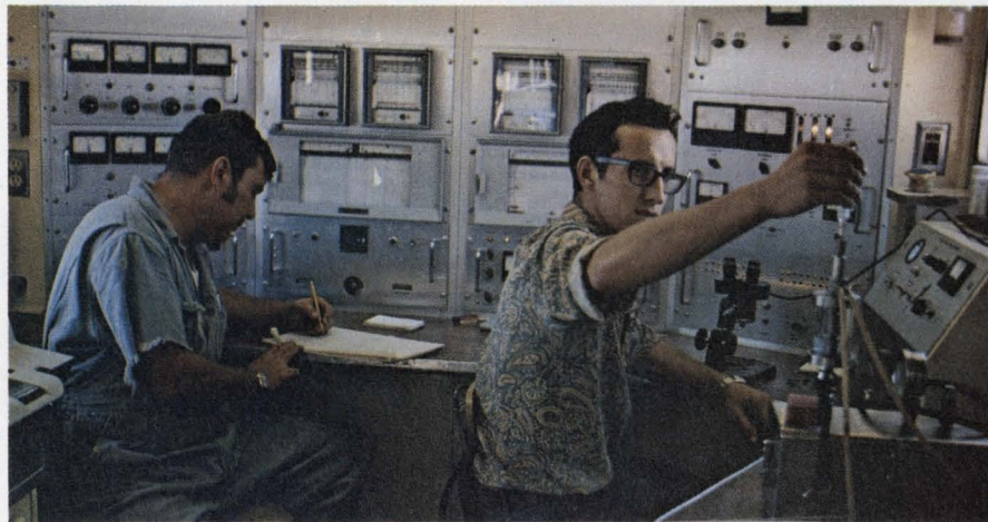
Data from transducers on the rig and from mud tests feeds into Baroid's Applied Drilling Technology van, parked alongside a well in South Texas. A two-man crew gives the driller geological and drilling advice.
