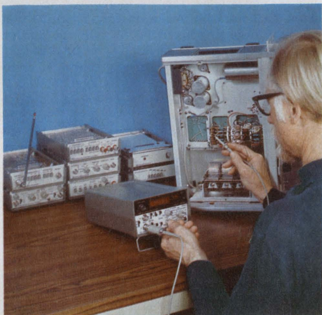
Snap-on, rather than plug-in, describes Hewlett-Packard's family of vertical-stacking modules. Units include counters, a counter-timer and a DMM/counter.
