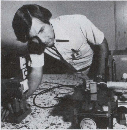
Test setup to measure the optical response of a laser prism modulator is adjusted by Martin researcher.
