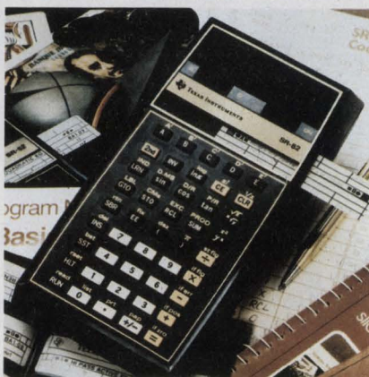
A complete 224-step program can be loaded from a small magnetic card into this TI SR-52 in two seconds.
