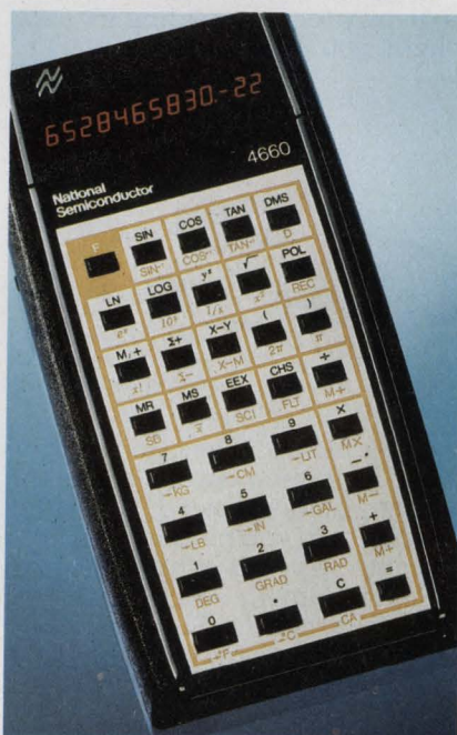
Metric-to-English measure conversions are a special feature of this National Semiconductor 4660 unit. It is totally programmed.
