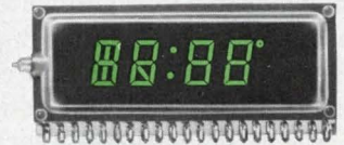
FG48D6 Dimension: 25.5(H)×56.5(W)×7(D)mm Character Size: 8.0(H)×4.2(W)mm
