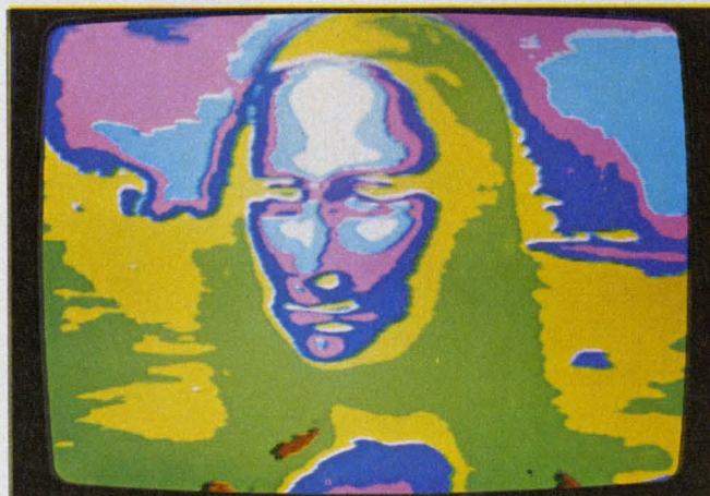
The Mona Lisa in eight grey levels and in eight-level pseudocolor (colors arbitrarily assigned to grey levels) demonstrate the capabilities of raster-scan graphics. The color image is produced on a standard color monitor.
