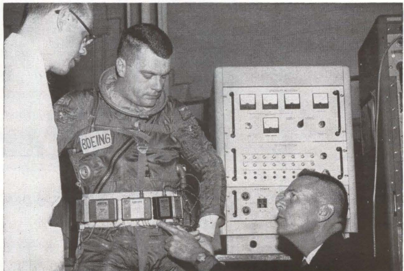
Miniature telemetry instruments, developed by Boeing for space medicine research, can be worn on belt, allowing subject to move freely. Arnoux Corp. will make the equipment
