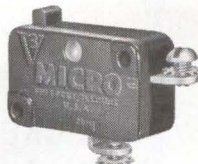
Screw terminals. SP-NC. 15 amps.
