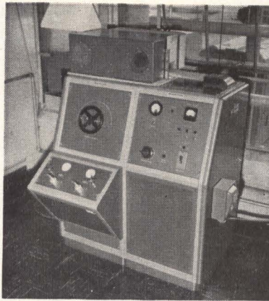
Sintering oven for Teflon sleeving incorporates some modifications to feed mechanism
