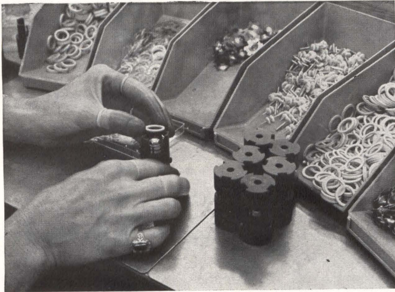
METALIZED-CERAMIC parts are assembled with metal parts in brazing jig. Many metals can be plated on the metalized ceramics and many types of metal can be brazed to the metalized ceramic
