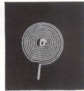
SPIRAL heater for a high power thyratron tube; 0.005 molybdenum coated with resist, the part ready for etching, the part after etching, and the final part ready for special coating
