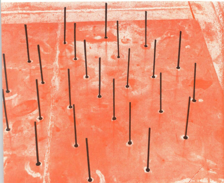
AMPLITUDE SCANNED circular array of concentric monopoles over a ground plane, University of Tennessee, Knoxville—Fig. 8
