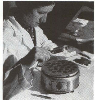
PROCESS has minimized rejects of disks subjected to microscopic inspection for flaking porosity and adherence
