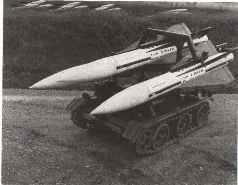
HAWK GUIDED MISSILES on mobile loader which carries missiles to launching site. Army's Hawk is built under Raytheon Company prime contract, is designed for surface-to-air-use
