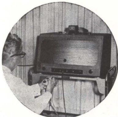
FILM READER scans data on 16-mm film. Seismologists can quickly locate events of interest but do not always agree on the interpretation of weak signals
