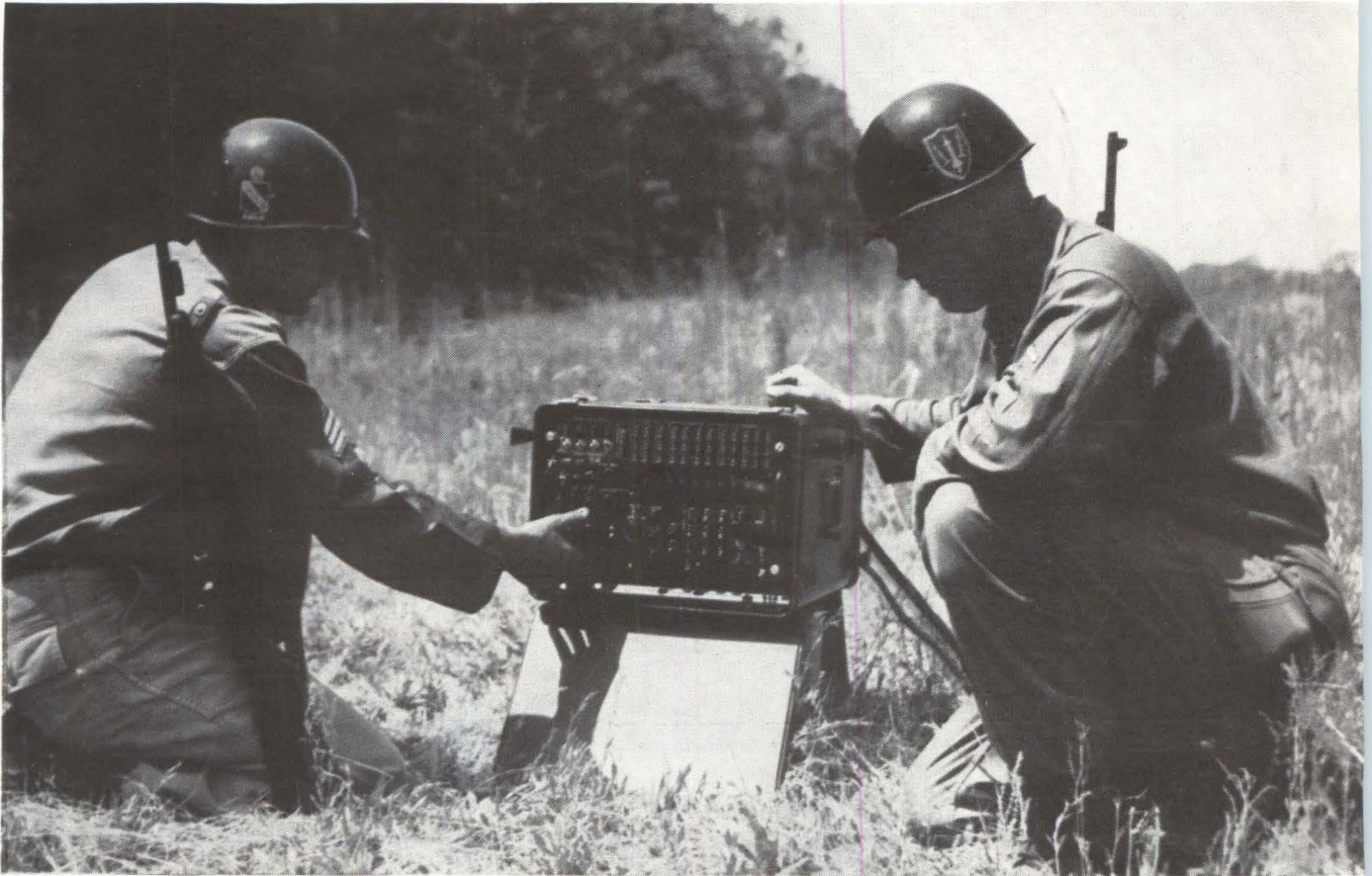
MICROPAC weighs in at only 90 pounds, but is a complete digital computer for tactical applications
