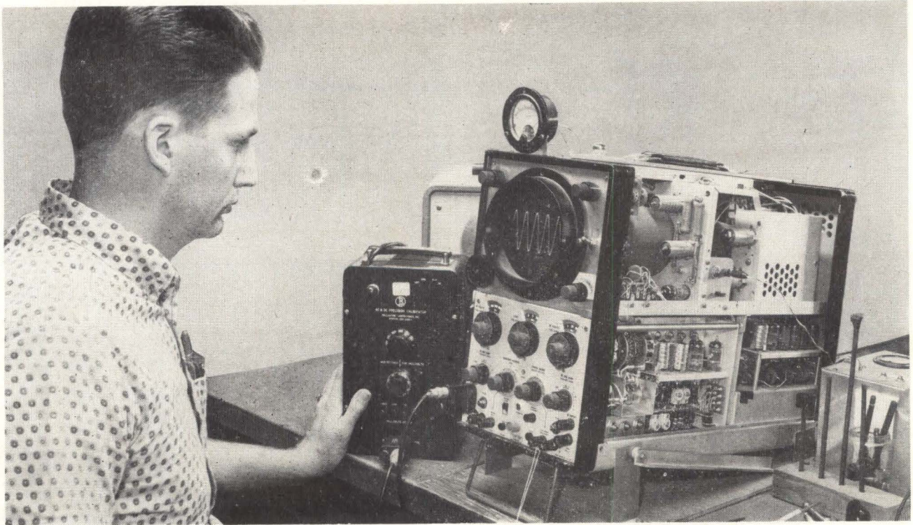
PRECISION D-C and A-C VOLTAGES are generated by Ballantine Laboratories calibrator (left) shown providing stable reference standard in oscilloscope calibration. Standards instruments and devices represent a maturing market
