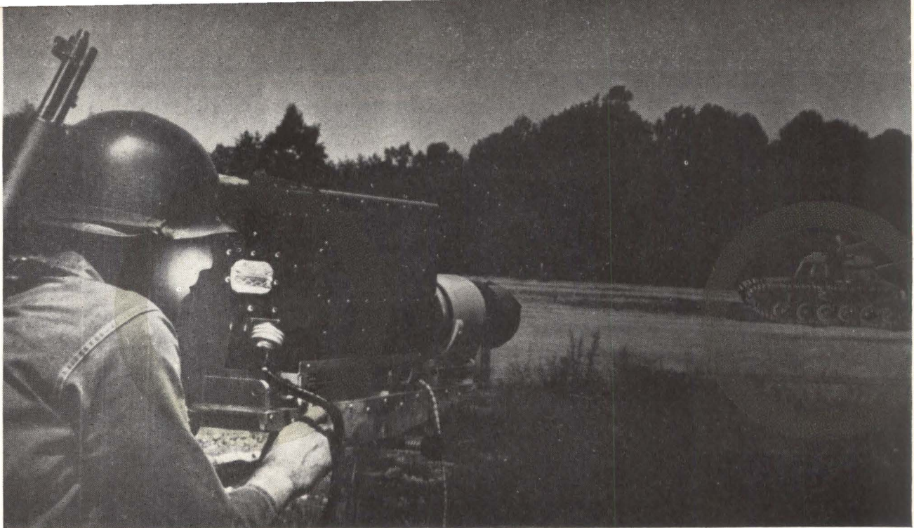
AMBIENT LIGHT SURVEILLANCE system for Army allows tv camera to view tank in the dark. Image intensifier at pick up requires only starlight, moonlight and skyglow
