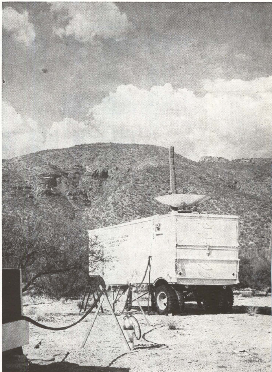
VERTICAL DISH used with coherent pulse doppler radar for cloud studies is mounted atop the mobile unit
