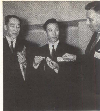
KLYSTRONS weighing 93 grams for use at 35 Gc are held by S. Aoi and K. Fujisawa, Oki Electric
