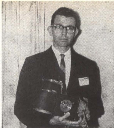
OSCILLATOR in Sperry's new line is shown by W. R. Day. Its range is 80 to 110 Gc
