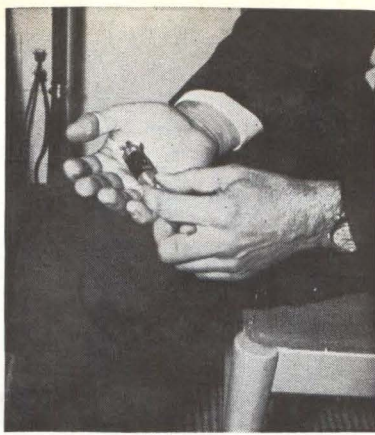
VARIABLE directional coupler from Amperex for 2-mm service has a 3 to 40-db coupling range
