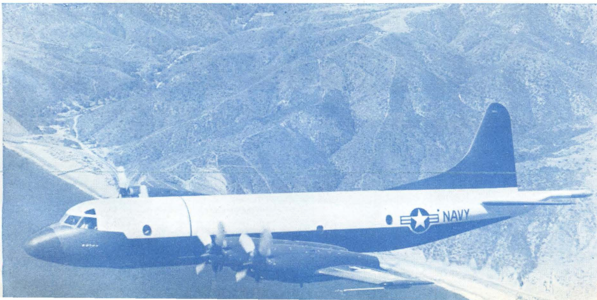
ASW PATROL PLANE, Orion, helped Navy track and flush Soviet submarines during the Cuban crisis. Extending from tail is magnetic anomaly detector
