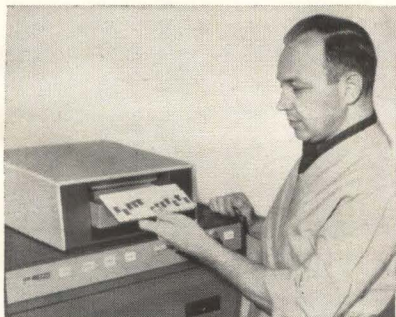
IBM 1030 Data Collection Units are installed anywhere you need them throughout your factory. Employee uses new IBM data cartridge to record information and transmit it to the central computer.
