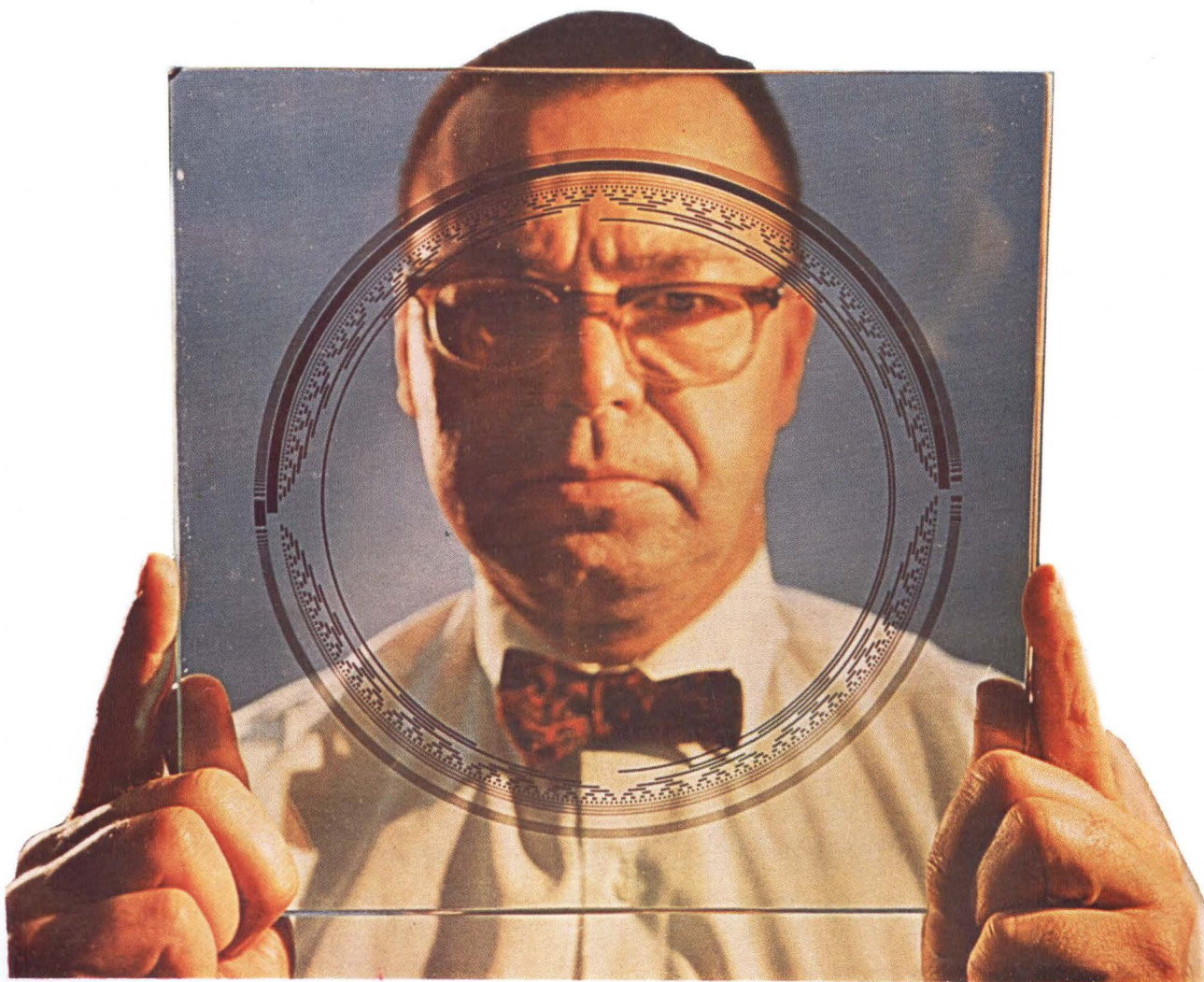
DISK ENCODER is photographically produced using a diamond-ruled master disk
