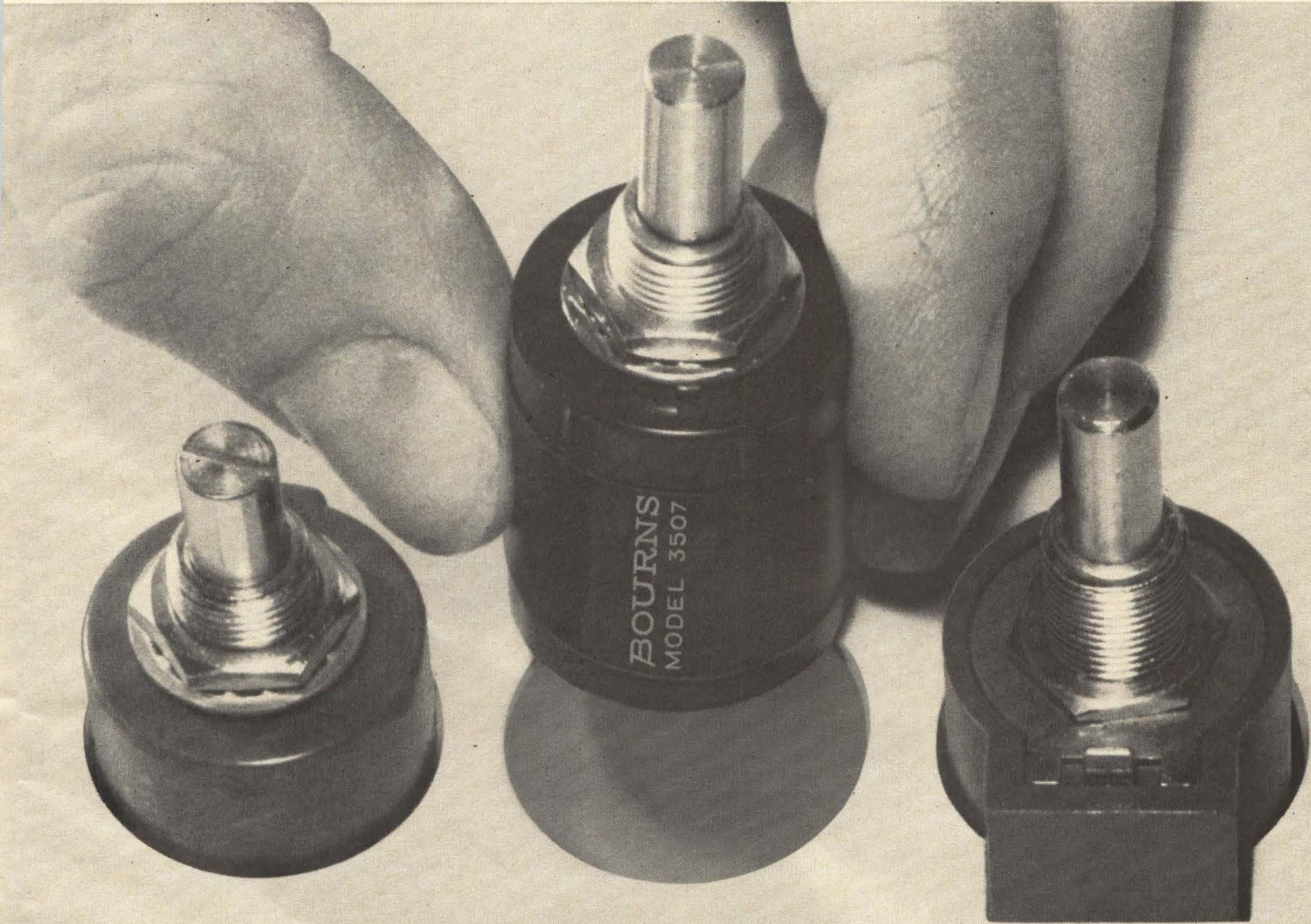
Mil Type Multi-Turn Precision Potentiometer
