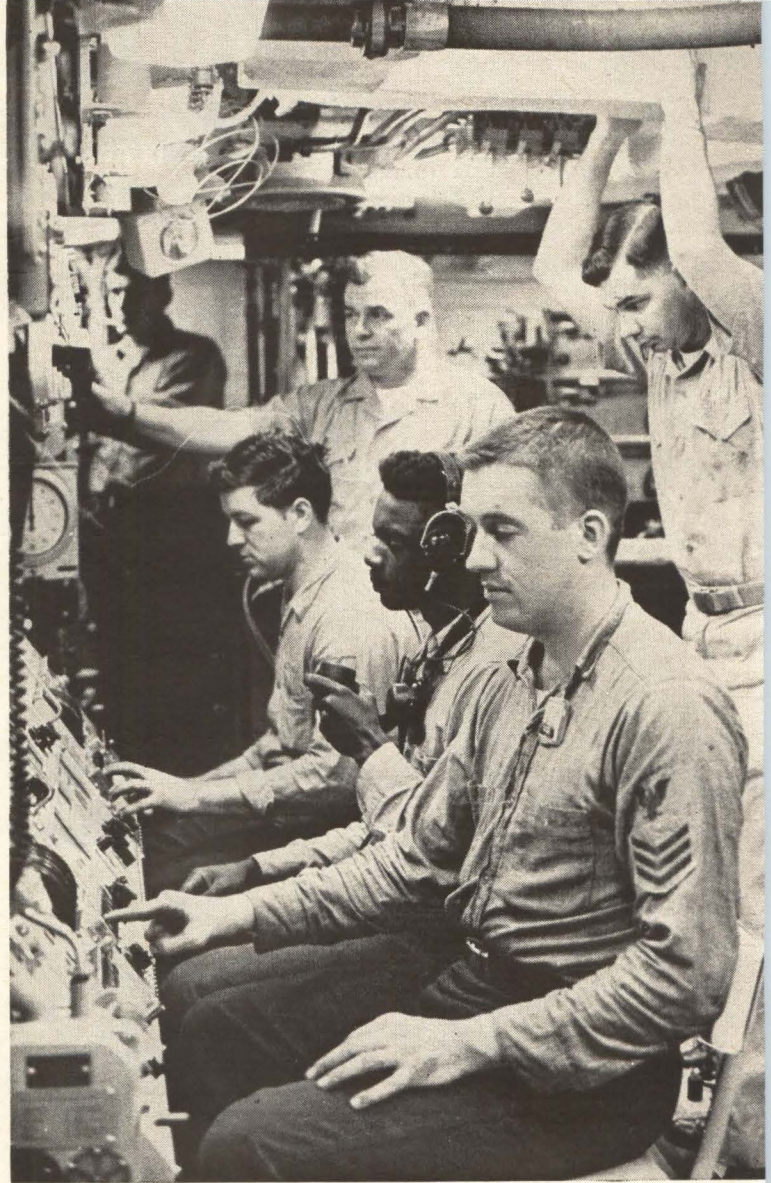
Weapons control panel in torpedo room. Each outboard torpedoman pushes buttons to prepare two torpedo tubes for firing. Torpedoman in middle fires the "fish." Weapons monitor locks out rest of firing cycle if prior events are not completed or occur out of sequence.
