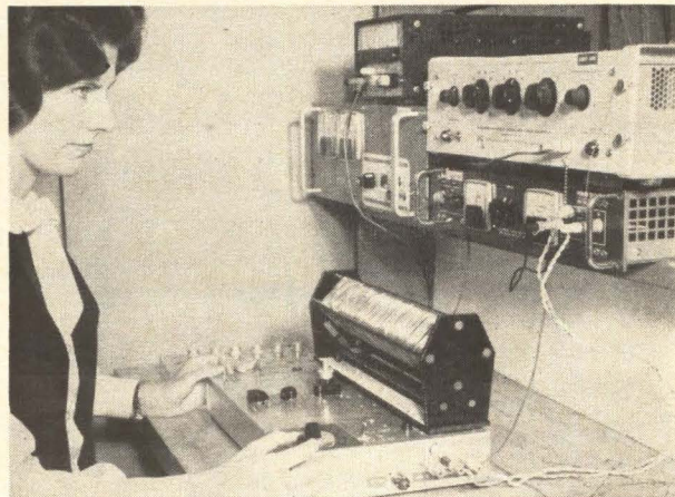
Collector current control is increased until second-breakdown oscillations are detected by reverse-biased second-breakdown test set.
