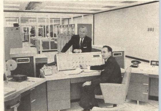
From the street, the control console of the General Motors "nerve center" looks like this. The system will eventually handle 100 million characters a day.
