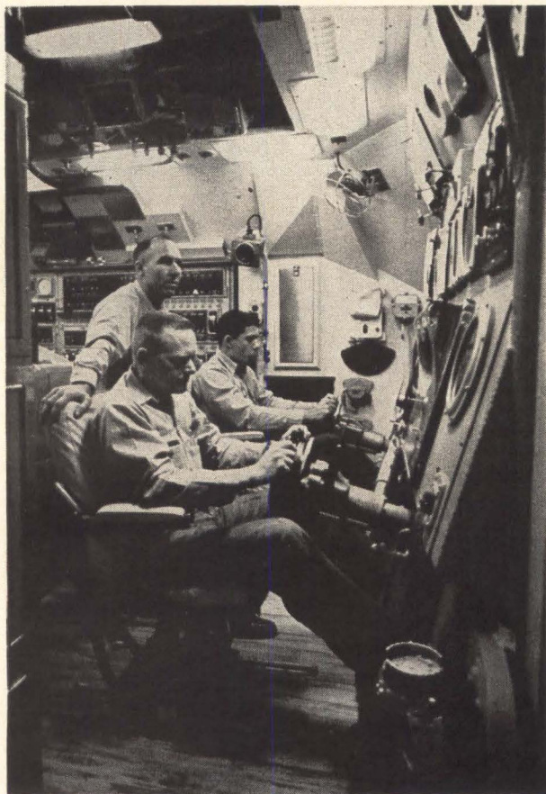
Control center of submarine. Sailor in foreground is helmsman or inboard planesman. He controls course, speed and angle of sail planes. Beside him sits the outboard planesman who controls the angle of the stern or main diving planes. The diving officer stands behind the planesman. Panel in background is ballast control, diving station of the Chief of the Watch.
