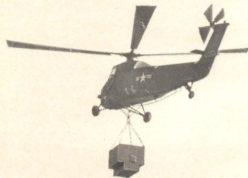
24-channel, dual-diversity, 1 kw tactical tropo terminal in S-144 shelter—total weight only 1500 lbs.
