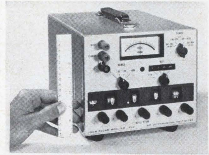
Model 871AB is a line-and-battery powered d-c differential voltmeter
