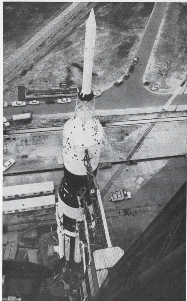
Saturn I launch vehicle is forerunner of the giant Saturn V booster that is expected to carry three astronauts to the moon by 1970. The Saturn I is shown during a radio-frequency-interference test prior to a recent launch at Cape Kennedy.
