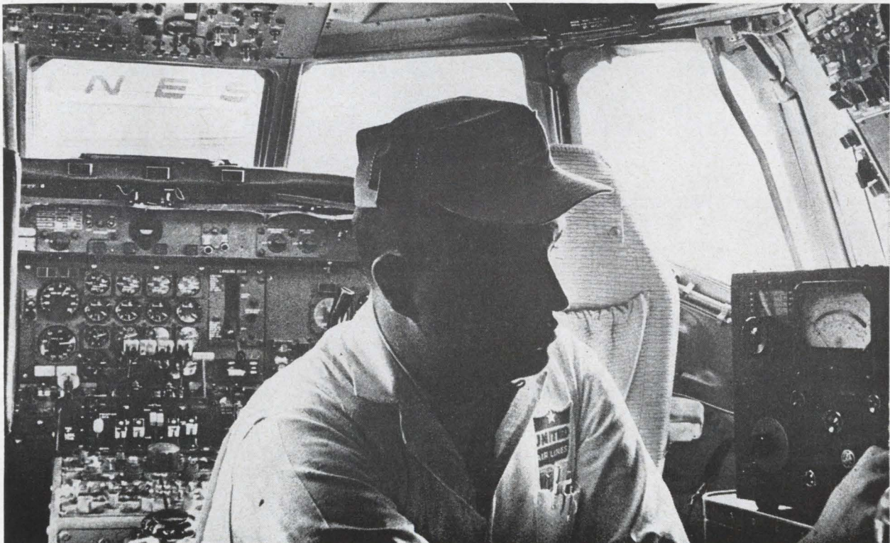
Test and maintenance of instrumentation used in commercial jet aircraft are carried out using an impedance-measuring instrument by Hewlett-Packard's Boonton Radio division.
