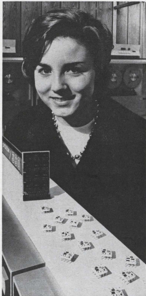
Core-memory at left (single plane in foreground) stores up to eight million characters, accessible in .000008 second, a major advance in IBM's system 360 computers. Another important feature, in photo at right, is the 360's hybrid microelectronic circuits, which combine thick films (passive elements silk-screened on a ceramic wafer) and discrete components (active elements such as transistor and diode chips, made separately and soldered to the wafer).
