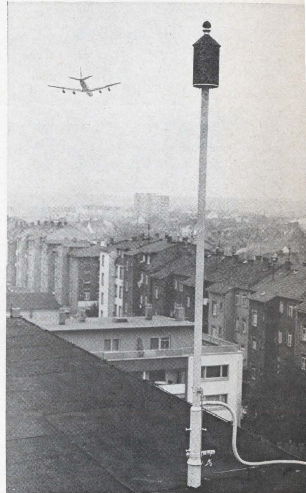
The roofs have ears in towns surrounding Frankfurt. This microphone picks up aircraft noise which is then analyzed to determine whether plane was off course, flying too low or too fast, or creating excessive noise in another way.
