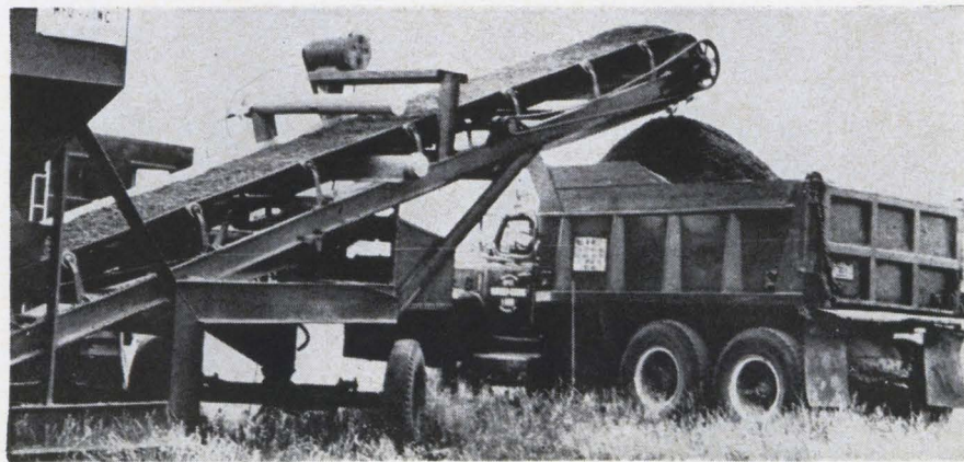
Gamma-ray weighing system for fill dirt used in road construction costs from $5,000 to $7,000. It is expected to cut road-building costs by $10,000 per mile.
