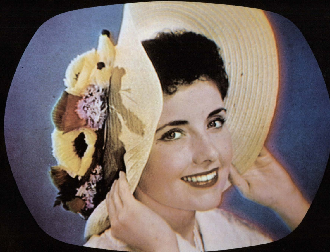
Single-sideband distortion causes color crosstalk.
