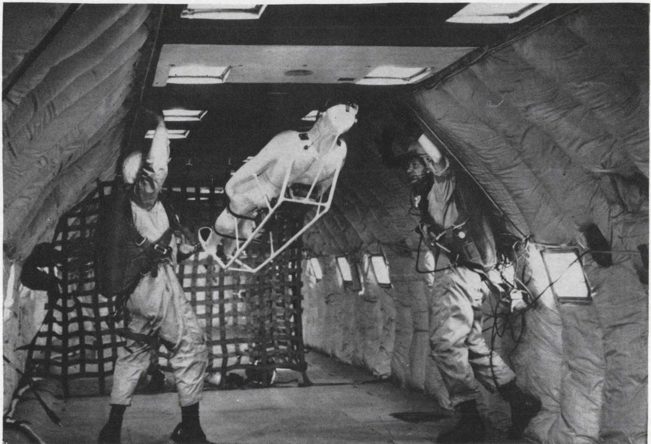
Instrumented couch is used to study a subject under zero gravity. In this experiment, by W.C. Hixson and D.E. Beischer of the Naval Aviation Medical Center, the free-floating couch provides an ideal way to obtain whole-body ballisto-cardiograph measurements.
