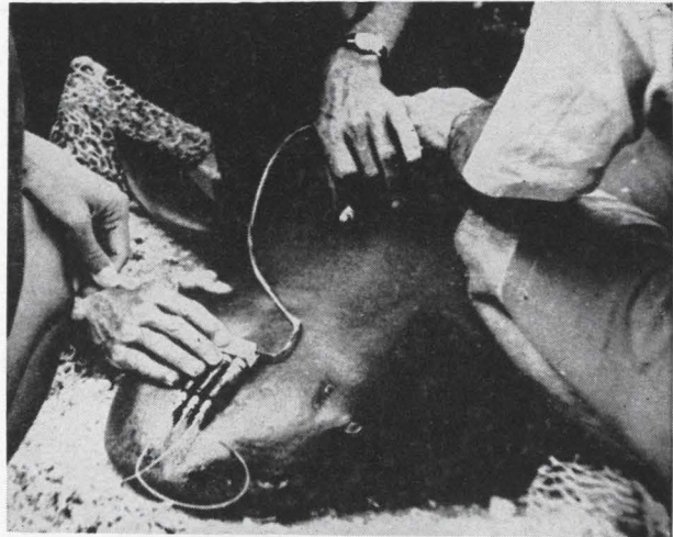
Tranquilized shark being equipped with a syringe assembly that will eject a chemical in front of the shark as it swims. The experiment, devised by H. A. Baldwin, at Cape Hays Marine Laboratory to study the effect of various odor stimulants on shark behavior, employs a two-way biotelemetry using ultrasound as the transmitting medium. Effect of EKG reaction to chemical is recorded remotely by transmission over a return ultrasonic loop.
