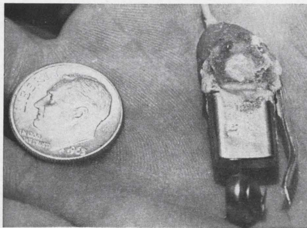
Small pack transmitter was designed by W. W. Cochran of the Illinois Wildlife Survey for tracking birds and small animals. It weighs 20 to 40 grams, depending upon battery size, and is attached to animal's collar. Parts for the circuit, a one-transistor crystal-controlled oscillator, cost $8 per unit.
