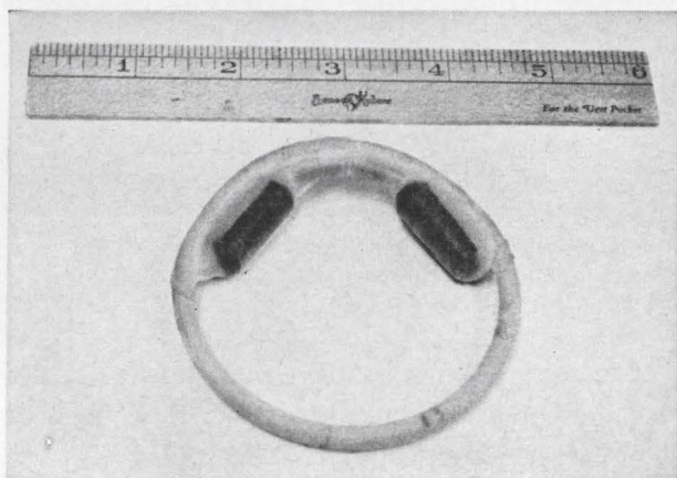
Low-power temperature-sensitive radio transmitter and its associated battery are inserted into the body in the rim of an arching domeless diaphragm. Designed by Dr. Alvin Singer of American Electronic Laboratories, Inc., it continuously transmits vaginal temperatures for up to six months.
