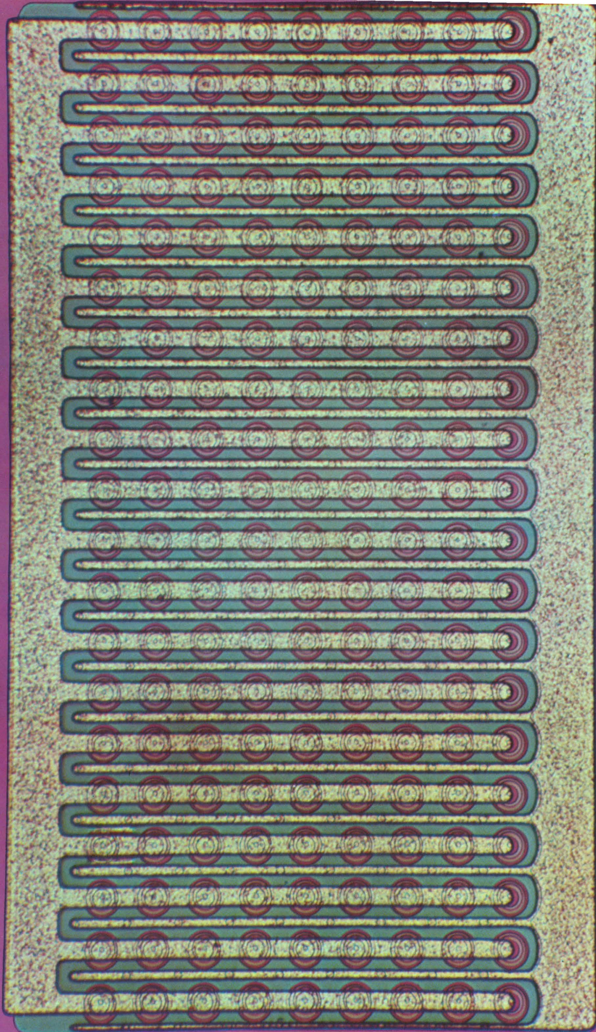
Overlay transistor has multiple emitters connected by an aluminum layer. This is RCA's TA2657, which has 180 emitters (small circles), each 2.5 mils in outside diameter. High emitter edge-area ratio gives power capability.
