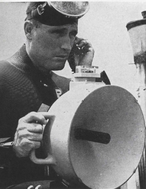
Berry L. Cannon uses the AN/PQS-1B sonar to search the ocean floor.
