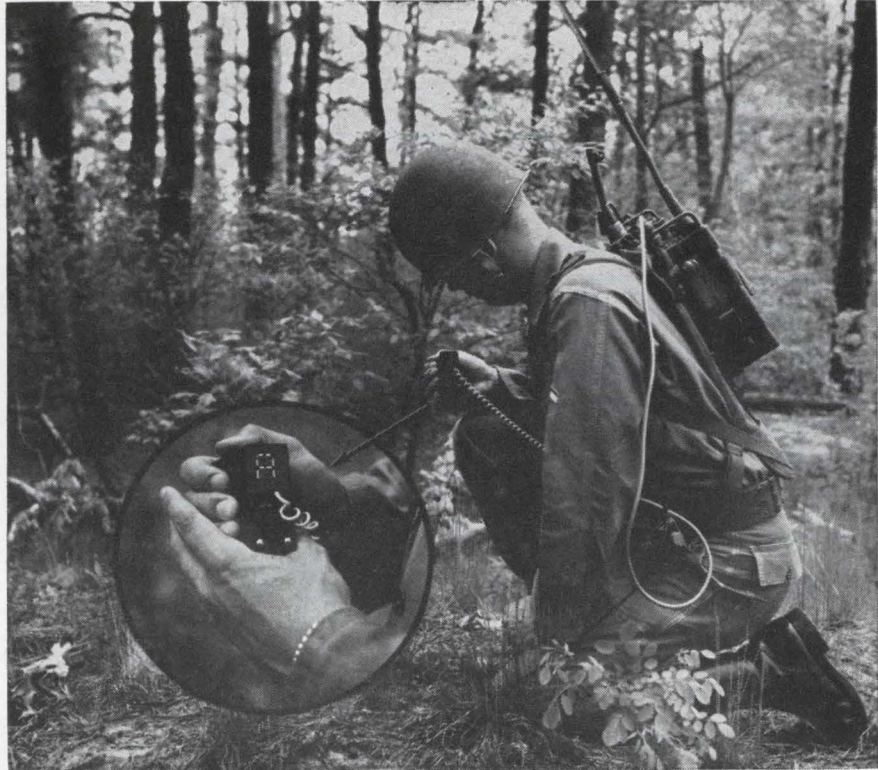
Morse code converter translates dot-dash-dot into letters.
