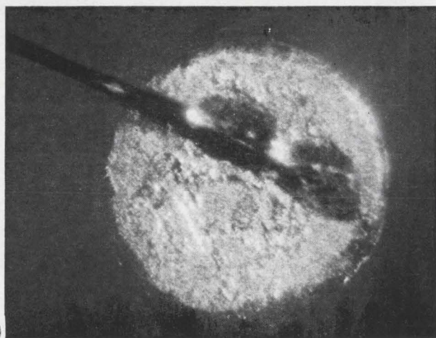
Aluminum bond made to top of a gold-plated post. Plague has formed, but not enough to destroy the bond.
