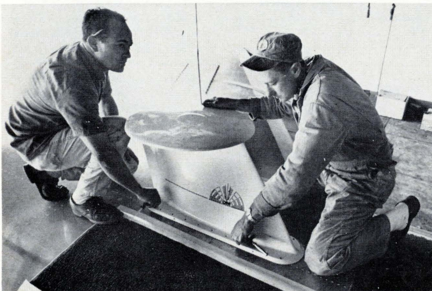
Winner. Disk-shaped antenna from Dorne & Margolin outperformed its competition in aircraft communications tests with the ATS-1 satellite.
