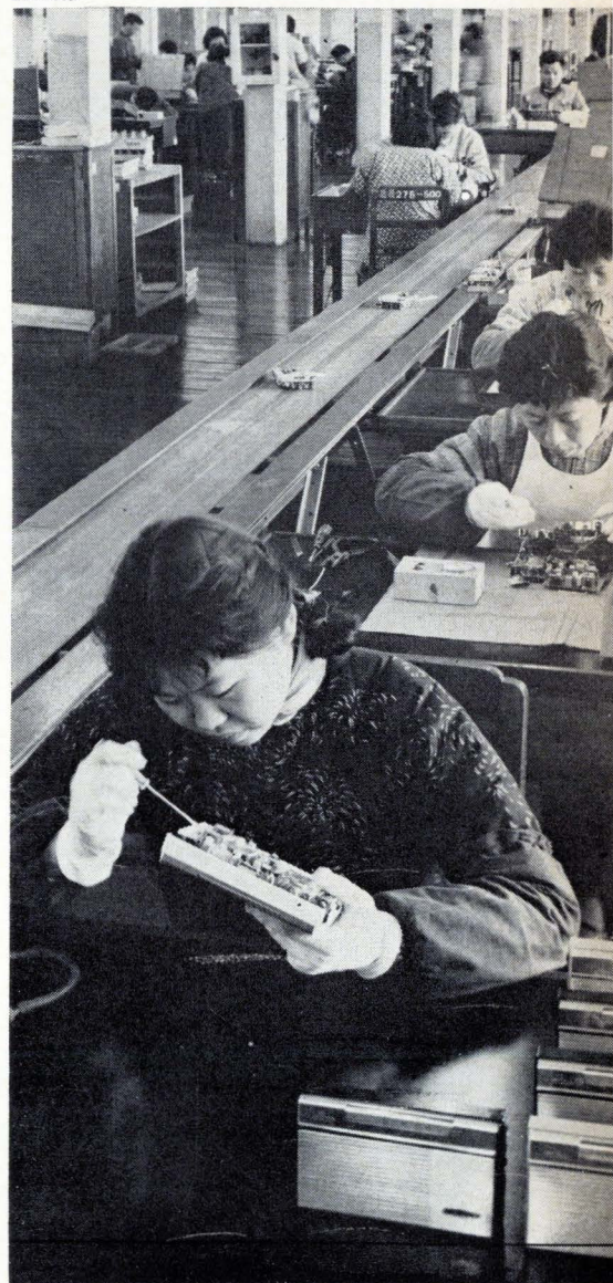
End of the line. Assemblers at plant in Shanghai put the finishing touches on transistor radios. Annual capacity is estimated to be 100,000 receivers.
