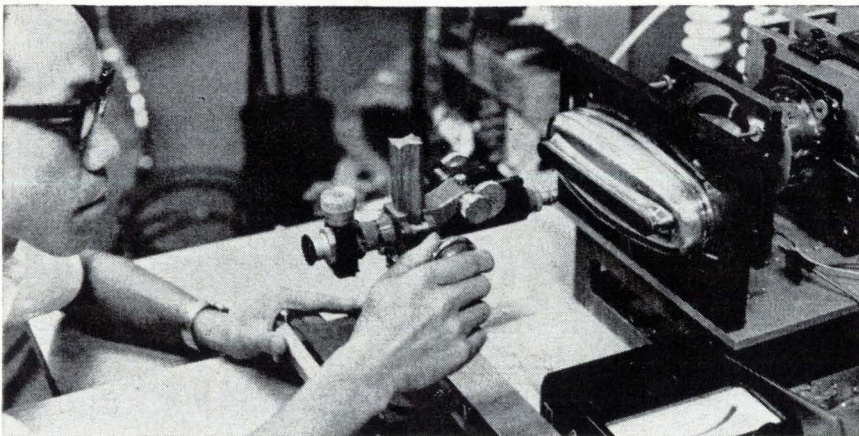
Checking fax. Engineer examines alignment of fiber-optic faceplate on facsimile receiver tube.
