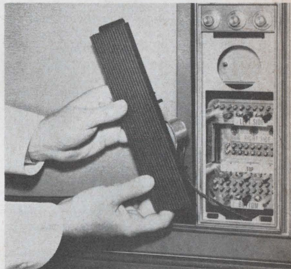
Voila. Zenith makes convergence panel easily accessible to the serviceman.
