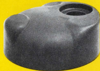
Stainless Steel 302; 7" diameter, .020" blank One draw • 10,000 psi
