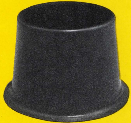
Stainless Steel 304; 12" diameter, .030" blank Two draws • 14,000 psi
