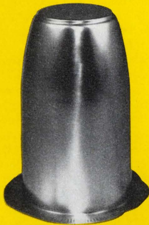
Brass 70-30; 12" diameter, .35" blank One draw • 12,000 psi
