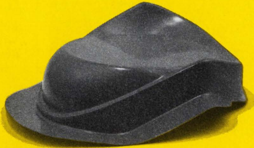
Aluminum 5257-0; 12" diameter, .035" blank One draw • 5,000 psi
