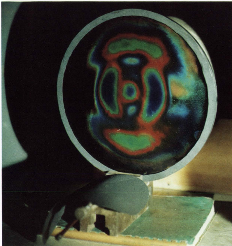
Radiation modes. The mode pattern appears on Mylar film coated with liquid crystals and placed in front of a radiating circular waveguide.
