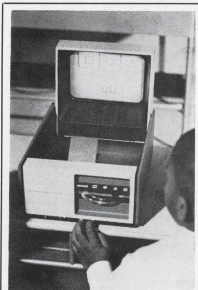
Teacher. CBS Laboratories and the Reading Institute of Washington, D.C., have developed this $350 programmed learning system, the AVS-10. Video—152 transparencies—line the outer edge of record; record has 600 lines per inch, plays at 22½ rpm. Response is 100 to 7,500 hertz. Slots on the cartridge operate microswitches to provide answers to questions.
