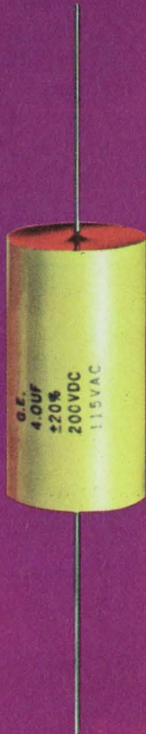
Polycarbonate Tubular Capacitors (left) 64 standard ratings. 100 and 200 volts d-c, 0.001 to 1.0 \mu\text{f} , -55 to 85C
