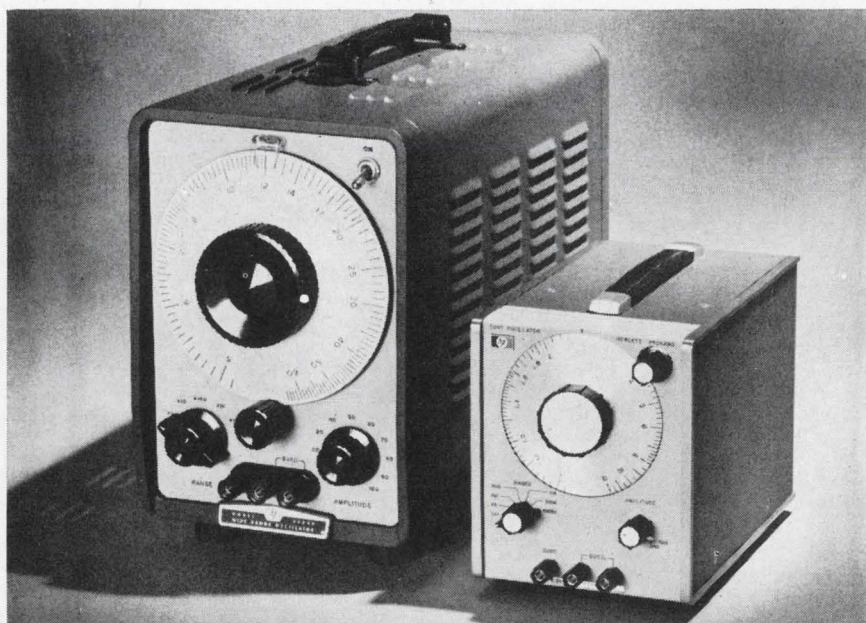
Old and new. Despite the gains of solid state design, about 20% of Hewlett-Packard's production is taken up with vacuum-tube instruments, like this wide-range oscillator, left. On right is H-P's solid state version.
