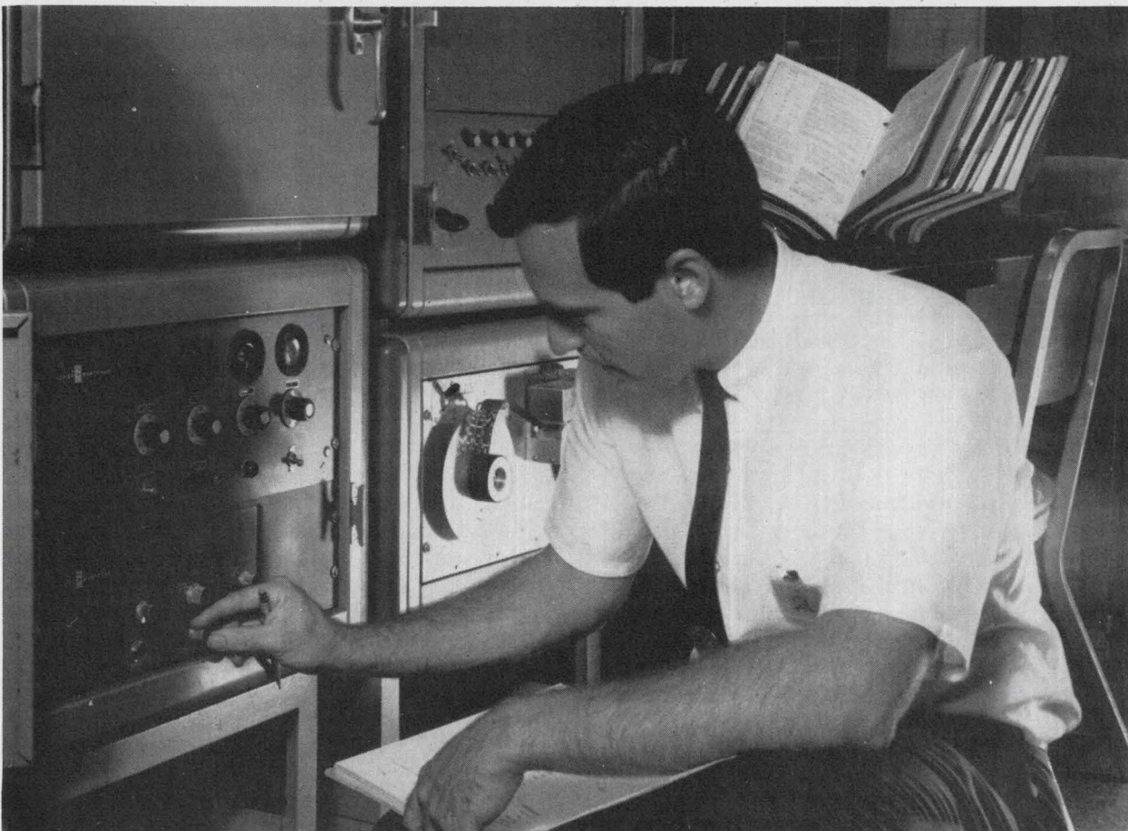
Voracious. Because control-system design requires tremendous amounts of data, this converter and paper-tape logger is sent to the field. Here the system is back at the hybrid center reading in tape for analysis.
