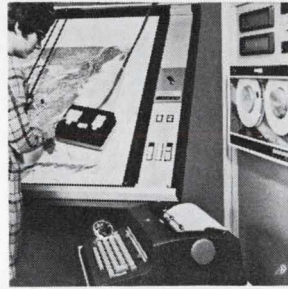
Digitizer 485 is an A/D device that can digitize both lines and points simultaneously. Features include whole value and incremental operating modes, a floating origin which permits starting point location to be anywhere on the tracing area relative to point or line coordinates, and a coordinate display that sums digitized increments. Calma Co., Kifer Road, Sunnyvale, Calif. [422]
