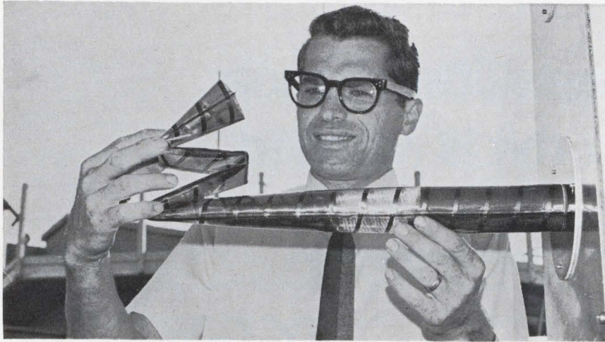
Folded up. TRW's pop-out helix antenna is planned for a communications satellite. Phased-array design has high gain and is lightweight. When satellite reaches orbit, plastic rods unfurl.
