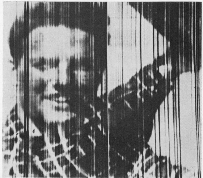
Crude proof. Although resolution and sensitivity are poor, RCA's early efforts with solid state image sensors proved the feasibility of a tubeless television camera.
