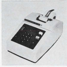
Adding machine model 708 is an input station for Data-Verter, a line of devices for recording manually on magnetic tape for subsequent computer processing. The unit has a non-add key that can be used to record non-add records e.g. reference numbers, dates, etc. It handles up to 10 columns of input and 11 of sub-totals and totals. Digitronics Inc., Albertson, N.Y. [423]
