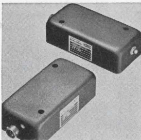
Charge amplifier type 1-308 is for use with piezoelectric transducers in general test lab applications. It operates on 24 v d-c at 7 ma and is protected against polarity reversal. Gain is 2 mv/pcmb. Frequency response is 5 to 10,000 hz \pm 5\% . Maximum shunt capacitance is 10,000 pf. Price is $95. Consolidated Electro-dynamics Corp., 300 Sierra Madre Villa, Pasadena, Calif. [381]
