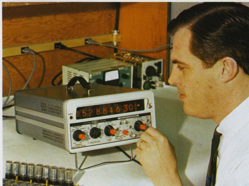
Checkout. Portable counter/timer 7035 is shown on a test bench, making a frequency measurement in the 500 Mhz band. In the foreground is one of the plug-in boards that combines the decimal count chains with the digital indicators. The board shows the extensive use of integrated circuitry that is characteristic of the instrument line.
