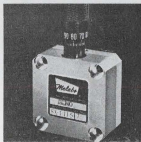
Bulk effect microwave oscillator SX-1 is a Gunn effect oscillator that can deliver more than 25 mw at any preset frequency in the 8 to 12.4 Ghz range. It is frequency and power stable over a temperature range of -30° to +71°C. The unit can be mechanically tuned ±500 Mhz from center frequency. Melabs, 3300 Hillview Ave., Stanford Industrial Park, Palo Alto, Calif. [403]
