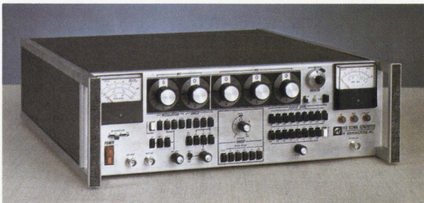
Locked in. The 808 uses an indirect technique—phase locking—to generate its output frequencies, which run from 50 kHz to 80 Mhz.
