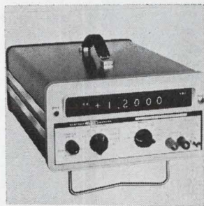
Dual slope volt/multimeters series 9200 feature \pm 0.01\% accuracy. They combine the best features of integration with provision for selectable input filtering to achieve a noise rejection of 80 db at 60 hz. The four-digit series also features automatic ranging and polarity, sampling speed to 6/sec and 20% overranging. Systron-Donner Corp., 888 Galindo St., Concord, Calif. [362]
