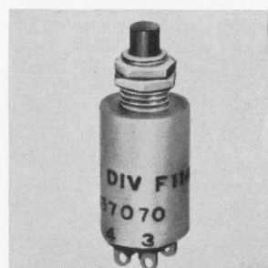
Double-pole, double-throw push-button switch B7070 is a snap-action device that measures 3/8 x 1 1/8 in. including terminals and pushbutton. Designed to meet the needs of data processing and industrial control, the unit has a minimum life of 50,000 operations at loads of 1 amp resistive or inductive at 28 v d-c or 115 v a-c. Controls Co. of America, Delmar Dr., Folcroft, Pa. [348]
