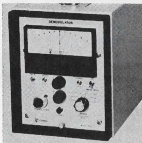
Exciter-demodulator model 7001, for use with all types of a-c operated electromechanical transducers, provides direct readout. Accuracy is 1.5% on any full-scale range; frequency response is from d-c to 100 hz with 1 khz carrier. Prices range from $450 to $650 and delivery is 4 weeks or less. Columbia Research Laboratories Inc., MacDade Blvd. & Bullens Lane, Woodlyn, Pa. [365]
