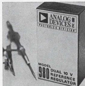
D-c reference source model 980 features output voltages adjustable for decimal or binary systems; remote sensing of the load voltage; shunt rather than series regulation circuitry for fast, transient-free operation and minimum interaction with the module's own d-c supply. Dual polarity is 10 v output at \pm 10 ma. Analog Devices Inc., 221 Fifth St., Cambridge, Mass. [386]
