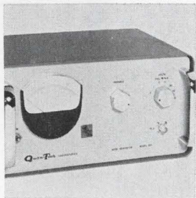
Random noise generator model 421 is designed to meet the need for an accurately calibrated noise source flat from 10 kHz to 12.5 MHz. To provide truly Gaussian amplitude distribution to better than 4 sigma and constant spectral density with frequency, the thermal noise of a resistor is used as the noise source. Quantech Laboratories Inc., S. Jefferson Rd., Whippany, N.J. [366]
