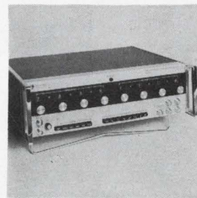
Programmable waveform generator model F280A is for use in automatic test system. Covering a frequency range of 0.01 hz to 1.1 Mhz, each unit can deliver up to 11 v peak-to-peak into 50 ohms in the manual mode or be programmed to generate up to 16 v p-p into a similar load (32 v p-p into open circuit). Data Royal Corp., 8014 Armour St., San Diego, Calif. 92111 [387]
