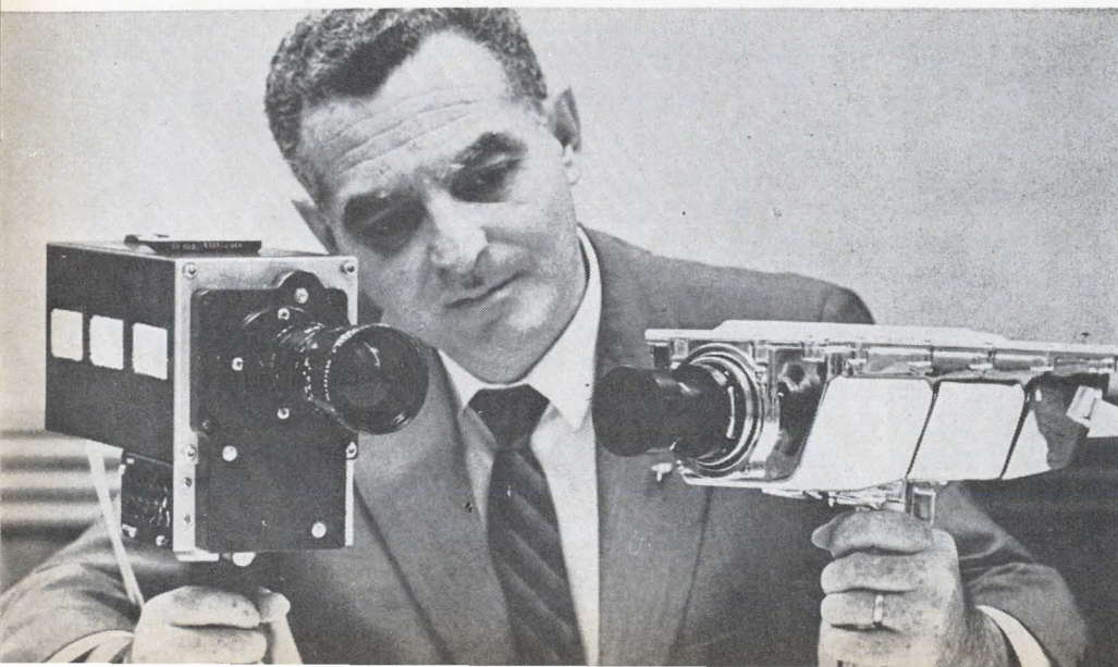
Space twins. Westinghouse's Apollo color camera, left, and the camera that took the pictures on the surface of the moon during the Apollo 11 mission use sec tubes developed for low-light-level tv applications.
