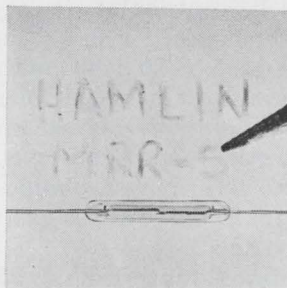
Magnetic reed switch MRR-5 is a single pole, normally open, Form A, and measures 0.130 in. max. glass diameter, 0.800 in. max. glass length, and 2.230 in. nominal over-all length, including leads. Initial contact resistance is 100 milliohms at 20 amperes turns overdrive. Maximum switching voltage is 500 v d-c; breakdown voltage, 1,000 v d-c. Hamlin Inc., Lake Mills, Wis. [345]
