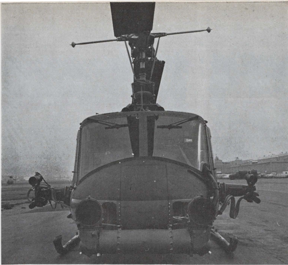
Dark eyes. Low-light-level tv and direct-view systems of Infant "see" through round light sensors mounted on front of this UH-1C helicopter. Targets can also be illuminated by searchlights mounted at sides of cabin. Hughes Aircraft developed this system for the Army's Night Vision Laboratory.
