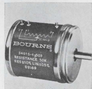
Servo mount precision potentiometer model 3451 is a 10-turn 2-in. diameter device featuring an Infrinon conductive plastic element. It has rugged element terminations, essentially infinite resolution, and a 50 million shaft revolution rotational life. Resistance range is 1,000 ohms to 500 kilohms. Power rating is 5 w at 70° C. Bourns Inc., 1200 Columbia Ave., Riverside, Calif. [344]
