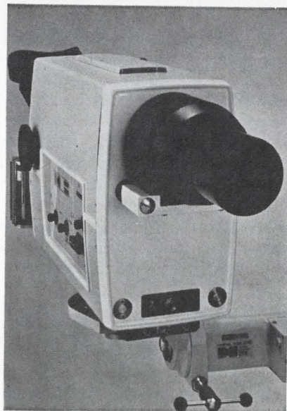
Greased lightning. Imacon high-speed camera uses controlled deflection of electron beam to capture 10 or more frames at 20 million frames a second.
