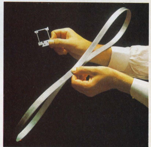
Small and light. Desktop-size printer swings open in front for loading convenience. Font belt, shown above with one of the print hammers, takes the place of chains and drums used in many printers.
