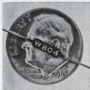
Wirewound power resistors in the WP line have a standard total resistance tolerance of only 1%. They are stocked in a variety of 9 sizes and styles ranging from 0.078 x 0.250 in. to 0.375 x 1.780 in. in ratings from 0.4 to 11 watts. Maximum resistance ratings are available from 3.5 kilohms to 200 kilohms. Nytronics Inc., 550 Springfield Ave., Berkeley Heights, N.J. 07922 [342]
