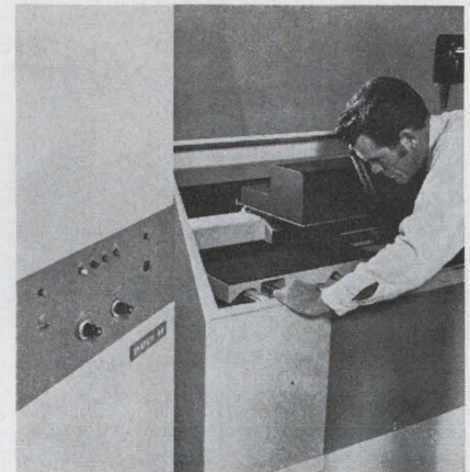
Artwork station. Photohead is mounted over plotting table. Light-proof cabinet forms a darkroom.
