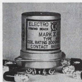
Relay series 600 (4pdt) is for aircraft, missile and ground support equipment power switching. It is rated at 10 amps for 100,000 cycles minimum at 28 v d-c. Its contact mechanism delivers a positive wedge-wiping action which cuts through surface films to create a continual self-cleaning of the contacts during make and break movements. Electro-Tec Corp., Ormond Beach, Fla. [346]
