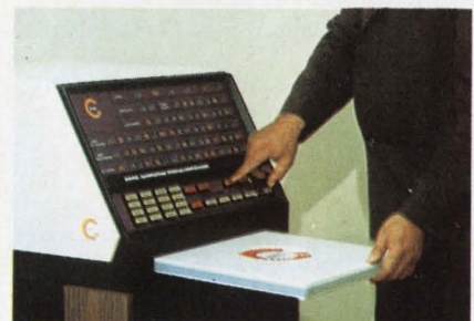
Air tight. Sealed cartridge containing disk is received or ejected at push of button on front panel.
