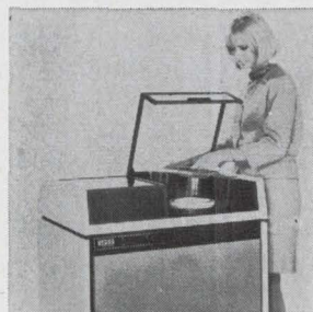
Eleven-high disk storage drive designated ISS714 has an access time ranging from 10 to 60 msec. It maintains complete disk pack and data compatibility with the IBM2314. The unit provides storage of 29 million bytes at a data transfer rate of 312,000 bytes per sec, and utilizes the 20 recording surface. Information Storage Systems Inc., N. Tantau Ave., Cupertino, Calif. [407]
