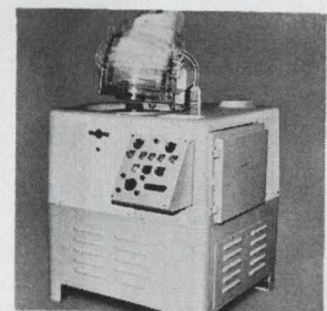
Automated wafer finishing machine simultaneously flat finishes both sides of silicon wafers, ceramic substrates and many other materials with surface finishes to one micron precision. One worker operating several machines can easily achieve production rates exceeding 1,000 high-precision 1-in. wafers or substrates an hour. P.R. Hoffman Co., 359 Cherry St., Carlisle, Pa. [424]
