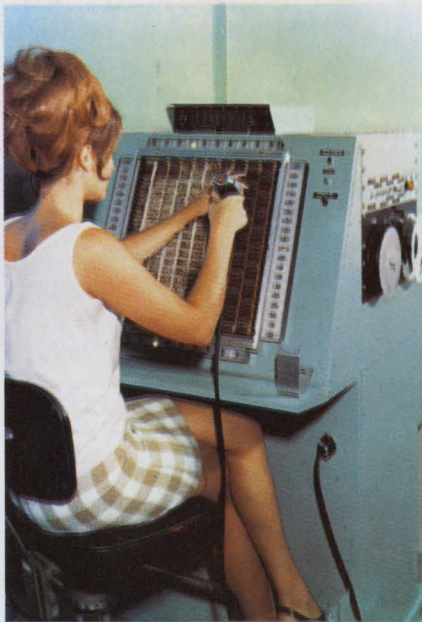
Philco-Ford Wiring Verifier virtually eliminates wiring errors. Design prevents wire wrap gun from operating if wrong pin is selected.
