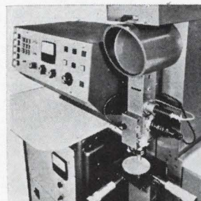
Universal laser system 202 is for production of semiconductor devices including IC design and fabrication. The solid state system has been successfully applied in effecting various changes in silicon wafers through precise irradiation. It permits a component to be made at a specific point on a wafer without disturbing surrounding material. General Laser Corp., Natick, Mass. [427]
