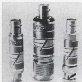
Broadband tunnel diode detectors series D cover the 1-12.4 Ghz range. They come with either type N or miniature inputs and are available with maximized sensitivity over octave or multioctave bands. Prices for the type N range from $75 for octave band coverage without a d-c return to $95 with integral d-c return. Electro/Data Inc., 1621 Jupiter Rd., Garland, Texas [407]
