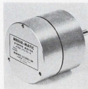
Stepper motor 2.75-100-1-8 uses a nutating disk principle. The disk has a bevel gear and is attracted by 8 solenoids. By varying gear ratios and switching sequences, from 200 to 1,600 steps per revolution may be obtained. Standard unit offers 800 or 1,600 steps/rev, 30 in. lbs of torque at stall, 5 in. lbs at 4,800 steps/sec. Mesur-Matic Electronics Corp., Warner, N.H. [367]
