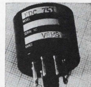
Solid state relay designated Mini-tactor model 751 is activated by a-c signals as low as 10 mv. It is suited for industrial, aerospace and military applications where environmental conditions, miniaturization or power conservation are required. It will switch up to 2 amps at 200 v rms. Price is $25 in small lots. E.D.C. Data Components Corp., Massapequa, N.Y. [348]
