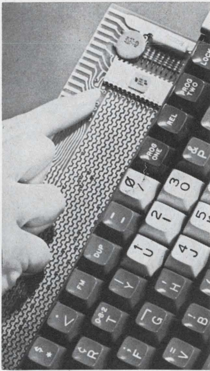
All in one. MOS encoding circuit replaces multitude of discrete components.
