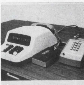
Data collection terminal DG-3 may also be used at the computer center to collect data off line. Data is received over the telephone from a remote DG-3 and is written off line on a computer compatible magnetic tape (7 track, 556 bpi or 9 track, 800 bpi). Data tape is then mounted on computer tape drive for processing. Applied Peripheral Systems Inc., Houston [386]
