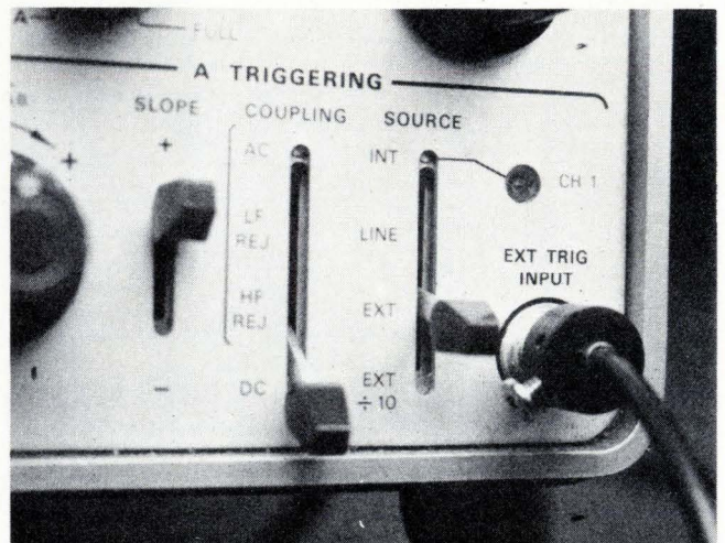
1. Modified. Optic trigger input in standard oscilloscope achieves high isolation in an electromagnetic environment.
