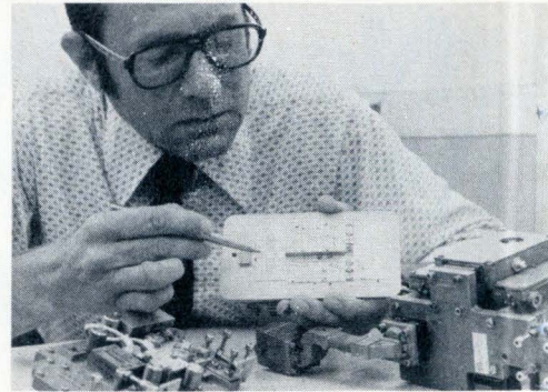
MARS is sophisticated. The tiny S band microwave microstrip IC replaces a large waveguide used in earlier radars.
