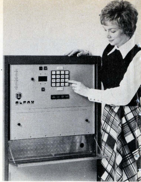
Detector. Microprocessor-based spectrometer makes drug tests automatically.
