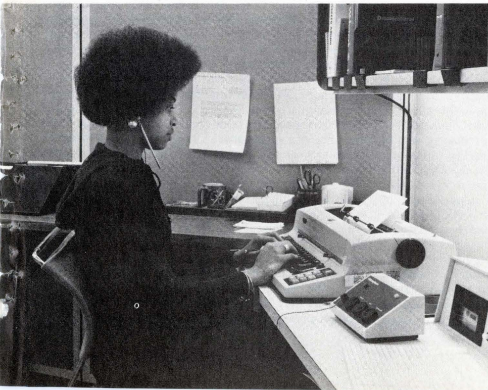
9. Thought control. Dictaphone's new Thought Tank System 193 provides the ability to set up a word processing center serving several correspondence originators with a centralized transcribing operation. Here a marketing manager at the company's Rye, N.Y. headquarters (top, left) dictates over the telephone-like mike to the thought-tank Word Controller console which monitors incoming and completed dictation. The Word Controller supervisor (above) can direct dictation to the correspondence secretary (left) from the console. Other administrative secretaries use individual thought tanks to handle short messages or requests, such as arranging travel reservations.
