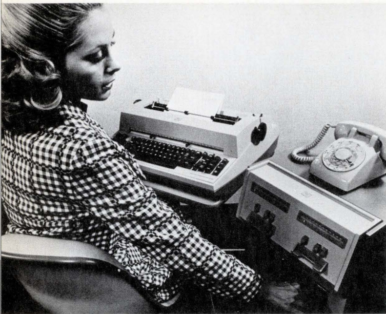
4. Typing by phone. Among the automated typewriters with communications capability is this Redactron unit. It performs information merging and editing using telephone-transmitted information. Advantage of system is ability to use data from various offices.
