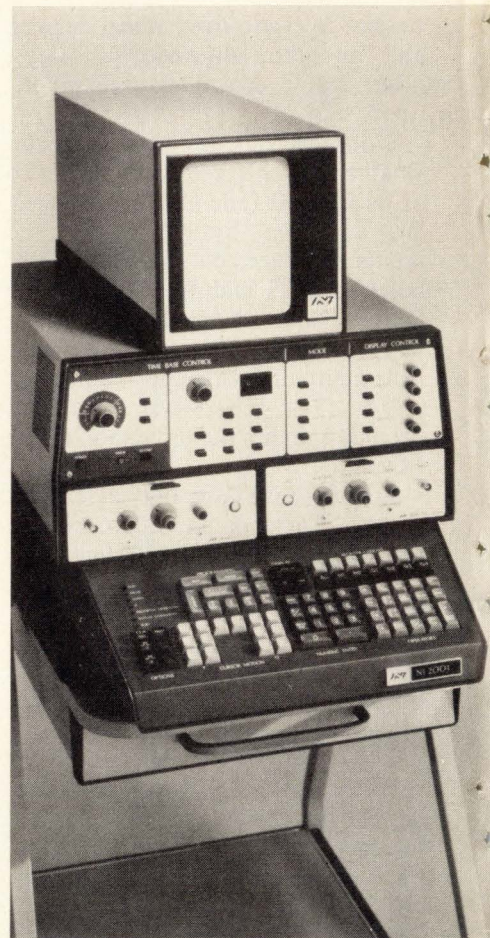
Bright scope. Special-function plug-ins for Norland's NI2001 programable digital oscilloscope will be slid into the panel areas just above the keyboard.
