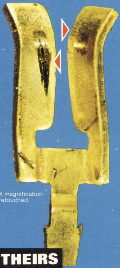
Arrows indicate scars and abrasions made by rough edge of lead frame.
