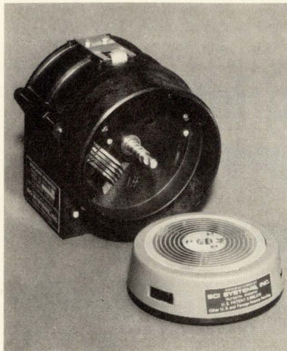
Here's the word. Print head, which pops into printer's plastic housing, writes one complete column at a time as paper, shown in real size, moves from right to left.
