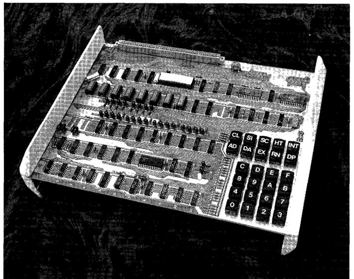
Western Data Systems has just introduced a new microcomputer card called THE DATA HANDLER. The card is based on the MOS Technology 6502 microprocessor.
