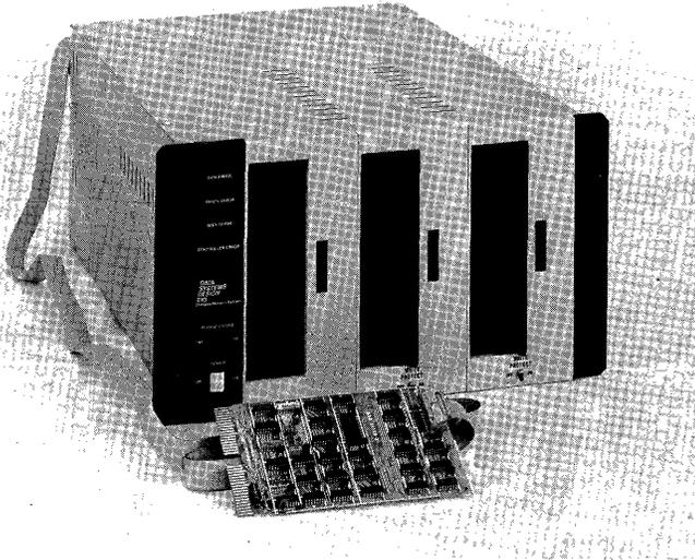
Data Systems Design's 210 Diskette Memory System is both DEC instruction set compatible and IBM 3740 format compatible. Diskette formatting and write protect are standard features of the unit. An 8-bit bipolar microcomputer controls all data transfers, monitors read/write head positionings, and performs data error checks. Self-test microcode verifies that the system is error free.
