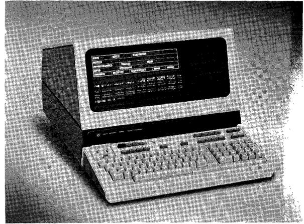
MSI's 3150 automatically generates 16 different character sizes, ranging from .111" to 1.776" high, or .095" to 1.520" high. It uses standard, pin-fed forms and prints an original with up to four copies (either carbon or carbonless). The printer employs a tractor feed, and its width is continuously adjustable to accept forms 4.0" to 14.875" wide.
