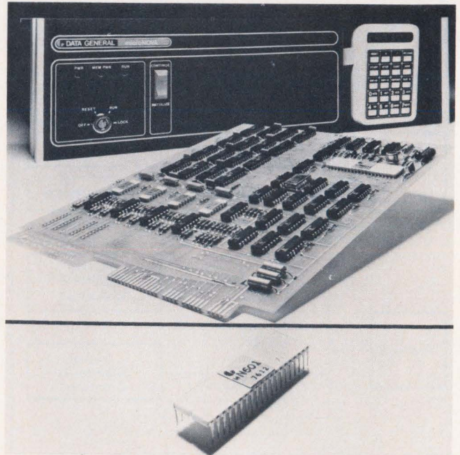
Data General's MicroNova microcomputer family is compatible with the Nova minicomputer architecture and supported by Nova software.
