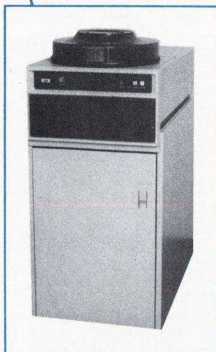
XEBEC 1700 STORAGE MODULE SYSTEM (300 MB for $27,500)
