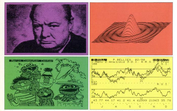
Graphics packages are the most popular serial-printer option and are becoming standard features. Printed by an Okidata Microline printer with a resolution of  $60 \times 66$  dpi, the images above are typical of the dot-addressable graphics available on matrix printers.
