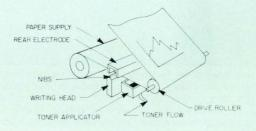
**Electrostatic** and **electrographic printers** are high-speed, non-impact devices using a moving row or rows of styli to charge spots selectively on dielectric paper. Toner is attracted to the charged area and then fused to the paper to create a permanent image.
