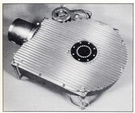
**Century's AMS 190:** Now being shipped in evaluation quantities, this 190M-byte 14-in. Winchester will be followed soon by a 380M-byte version. Ultimately, Century plans to bring the drive up to 1G byte using thin-film read/write heads. Note linear voice-coil actuator (l.).
