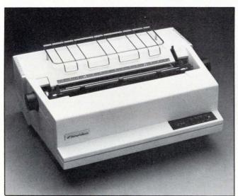
**Fig. 2. The DPS-55 operates at 55 cps** with a plastic print wheel, and, at 62 dB, is one of the quietest daisy wheels available.
