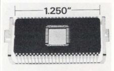
has a 100-mil pin pattern for soldering to a circuit board. Features include hermiticity to 1 × 10<sup>-8</sup>, low-temperature frit-seal lid and aluminum wire-bond fingers. Planarity of bond fingers meets or exceeds requirements for automatic wire bonders. DIP configuration permits use of existing assembly and transport equipment. The package is also available in 64- and 40-lead models. **Diacon, Inc.**, 12810 Hillcrest Rd., #209, Dallas Texas 75230. **Circle No** 390
