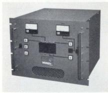
power. The internal battery charger has an automatic float-equalize circuit for charging after a utility failure and consequential battery discharge. Price is \$3125. Nova Electric Manufacturing Co., 263 Hillside Ave., Nutley, N.J. 07110.
