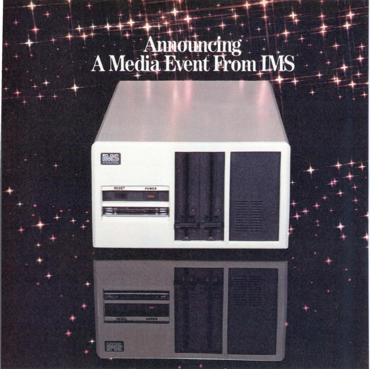
Configuration shown includes two slimline double sided, double density drives, 40 M byte Winchester subsystem with tape back-up
