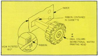
Impact-matrix printers have symbols that are composed of a series of dots. A set of needles in the print head strikes the printer ribbon to form the character.
