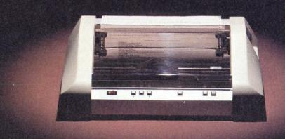
Since their introduction in mid-1980, the Anadex highresolution DP-9500 Series matrix printers have set new standards for printer quality and performance. All models feature the rugged Anadex 9-wire print head that combines long life with resolutions of 72 dots/inch vertical and up to 75 dots/inch horizontal. With this kind of resolution, fineline graphics (under data source control) and razor sharp characters are pluses built into every printer.
