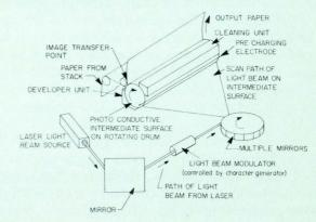
Photoelectrographic printers are high-speed, non-impact devices using light from a photographic drum or belt, or laser beam, to create a latent image of charged dots. The image then captures a dry toner that is transferred to plain or specially coated paper.
