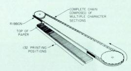
Chain printers operate on a principle similar to that of train printers, with the following differences: slugs on a chain printer are linked together, do not slide in a track and are driven by a sprocket wheel rather than a drive gear. Chain and train technologies are often combined, producing a more precise vertical character alignment.
