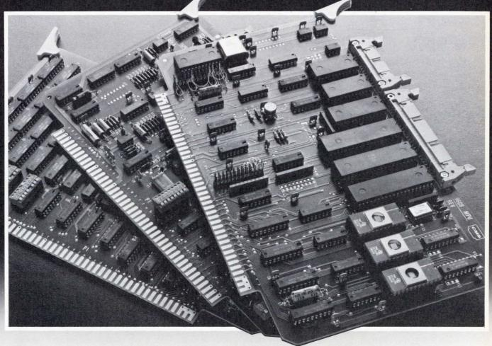
Creative Micro Systems is proud of its line of general purpose microprocessor support modules. These M6800/M6809 based modules are pin and outline compatible with the industry standard EXORciser\* and Micromodule\* bus.
