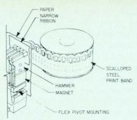
Belt and band printers employ either of two horizontally rotating devices: a belt with character slugs or a steel or plastic band with embossed characters. As the character to be printed moves into position, a print hammer is actuated, impacting the paper against the ribbon and the character.
