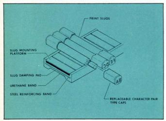
Cross section of Charaband, a blending of band and train technologies, used in Data products Corp.'s 2550 line printer, shows ease with which type caps can be replaced for special fonts or maintenance.
