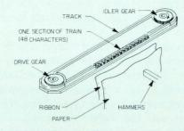
Train printers have character slugs with embossed character images that are pushed along a horizontal track by a pair of gear drivers past hammers that strike the paper and inked ribbon. Multiple sets of characters are typically in the track; therefore, only a fraction of a revolution is required to set a character in front of a column. The smaller the character set, the faster the printer speed.
