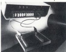
ated throughout with carbon black, rendering it electrically conductive without metallization. The film conducts electricity with a volume resistivity as low as 0.36 ohm  $\times$  cm. The moisture-proof film is stable
