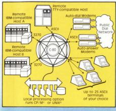
Dual IBM host interface ports allow simultaneous access to two totally separate host mainframes or networks. And, you're not limited to dialing in to the host; you can dial out to the public DDD network or you can dial out to the timesharing and electronic mail service of your choice.
