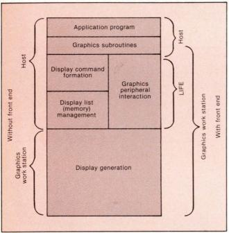
Fig. 2. Front-end processor at the graphics work station assumes control of display command function and memory management, freeing the host computer for other tasks.
