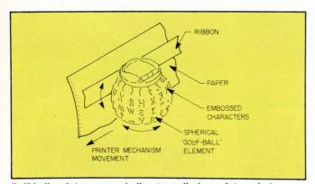
Golf-ball printers are similar to cylinder printers but use a spherical print mechanism. When the character has been rotated into position, the sphere strikes the paper.
