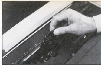
Convenience features are making serial printers more at home in office settings. The 25-cps Diablo model 620 offers drop-in plastic daisy wheels with automatic ribbon and print-wheel positioning. An electronic encoding system senses the wheel position after it has been inserted into an envelope-like enclosure and locks it in place.
