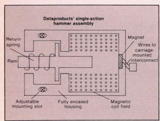
Figs. 3 and 4. Single is simpler. The single-action hammer assembly (I.) in the DP-55 is simpler and quieter than a conventional assembly (r.). In the DP-55 assembly, electrical impulses to the coil fire the ram into the print wheel electronically, with no intermediate striking action. The spring and
