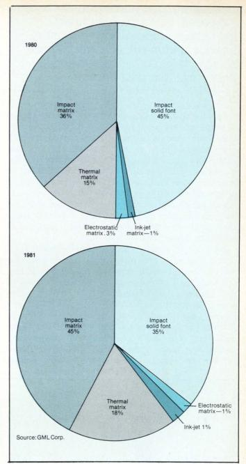
Fig. 4. Teleprinter technology is moving toward matrix methods and away from solid fonts. Matrix printing is gaining popularity in impact and non-impact applications because it produces high speed-to-price ratios. Solid font printers produce better quality output at slower speeds, but matrix printer resolution is improving daily.
