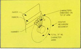
Daisy-wheel printers have a series of "petals" radiating from the hub of a wheel. Each petal has an embossed character, which is struck by a hammer after it has been rotated into position.
