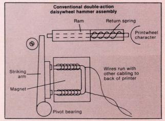
magnet assure minimum recoil of the ram. In the conventional hammer design (r.), there are two distinct firing movements: magnetic pulse pulls the striking arm into the ram, which, in turn, fires the ram into the print wheel, and produces the noisy "click-clack" sound typical of this design.
