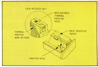
Thermal printers are non-impact printers that form characters by pulsing elements of the dot matrix on a special heat-sensitive paper. The heads are made from a high-resistance material, such as tin oxide or a semiconductor. Semiconductor heads are sometimes ICs that include decode and drive electronics in addition to the dot-matrix mechanism.
