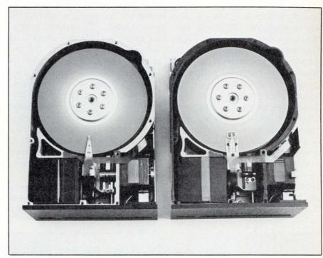
**Production of Seagate Technology's 12M-byte ST-512**, the first 5¼-in. Winchester to be equipped with thin-film read/write heads (r.) has been deferred in favor of the ST-412, a 12M-byte device incorporating manganese-zinc ferrite heads, like the ST-512 and the company's 6M-byte ST-506 (l.), the new drive stores data on two platters. The new drive is scheduled to go into production this quarter.
