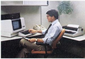
Digital's personal office computing option comes with a Z80-based CPU, dual mini floppy drive standard (second dual floppy drive optional), diagnostic disk, user documentation and guide, and installation hardware.
