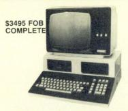
NEW! Industrial quality 6809E-driven microprocessing system for data processing, development and industrial control applications. Standard features include programmable video and communications, 600K bytes diskettes, 12' high resolution monitor, text editor, O/S and interpreted and compiled BASIC. Fully implemented IEEE-488 controller optional.
