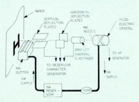
**Ink-jet printers** use electrostatic deflection plates to control a spray of electrically charged ink on ordinary paper. As many as 500 dots make up the ink-jet matrix, resulting in a close resemblance to solid character copy. A variety of fonts can be stored in additional ROM and switched in when desired.
