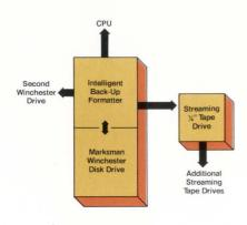
The formatter permits independent communication among all its interconnects: From disk to tape. Tape to disk. Or either drive to and from the CPU.
