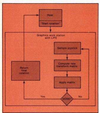
Fig. 3. Graphics manipulation of an object on the screen by joystick is performed at the work-station level.
