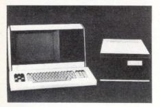
CTW-300. The series includes a selection of 5½-in., 10M-byte Winchester-disk drive, a 380K-byte dual minifloppy-disk drive or a 17M-byte tape-cassette drive in any combina-
