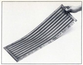
Print bands are etched from large sheets of stainless steel, separated, butt-welded and polished. Documation's bands are typically 58 in. long and contain 432 characters.
