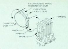
Drum printers have a complete character set for each column in a line embossed on a cylindrical steel drum. The surfaces are rotated vertically, using bearings at each end. Images are transferred to the paper when hammers strike both the paper and the inked ribbon, which are sandwiched between the drum and a bank of hammers—one for each column.
