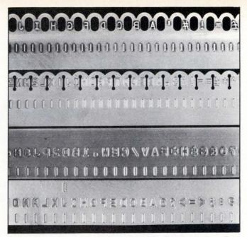
Various print bands are manufactured in America today: From top: Dataproducts' B300 and B600, STC/Documation's/3000 and Control Data Corp.'s 9380 family. The vertical bars beneath characters are timing makers. The thickness of Documation's band varies from 4/1000 to 6/1000 in. Characters are raised 19/1000 to 12/1000 in.
