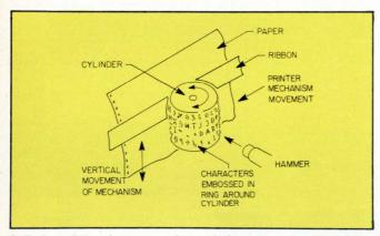
Cylinder printers have an embossed character set arranged in a series of rings around the cylindrical printing mechanism. The cylinder is rotated and shifted up or down to move the character into position and then a hammer strikes the cylinder.
