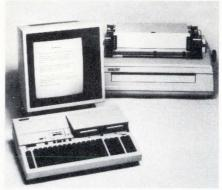
includes a 15-in. black-and-white display, a letter-quality printer and two built-in 3½-in. floppy-disk drives. A high-speed printer, 55-cps office-quality printer and a 40-character LCD are optional. Sony Corp. of America, Office Products Division, 110 E. 59th St., New York, N.Y. 10022. Circle No 370
