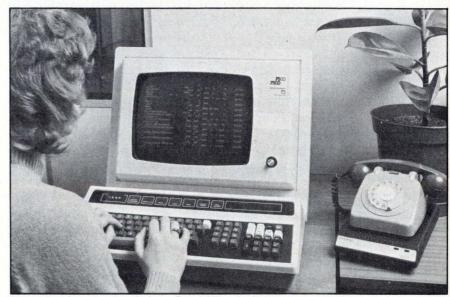
Planet local-area network from Racal-Milgo includes the terminal access point (under telephone), which can link one or two RS232 devices to the other devices on the ring network.
