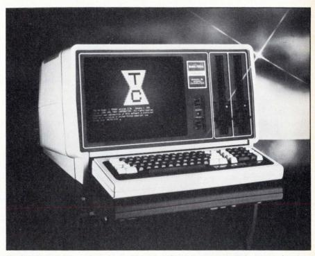
Tandy's first 16-bit  $\mu c$ , based on a Motorola MC68000  $\mu p$ , can include as many as three terminals, and can be expanded for a total of 512K bytes of memory.
