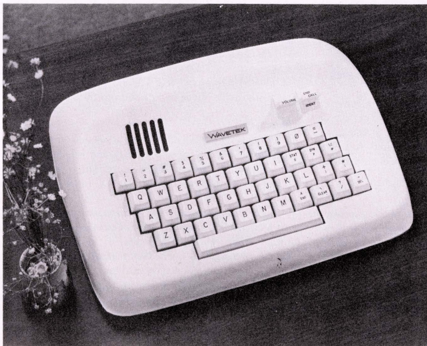
This touch-tone terminal includes a full alphanumeric keyboard. The built-in speaker for the audio response system can be seen on the upper left portion of the unit.
