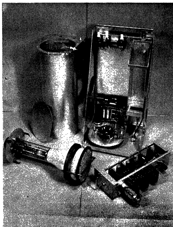
Figure 4 (right). The component parts of the cathode-ray tube storage unit
