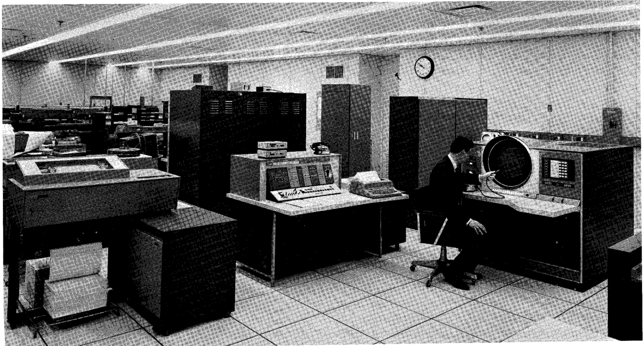
Figure 4. The IBM 1620 Mod. II Data Processing System, coupled to an IBM 4554 Video Display Unit, used to implement the automated logic partitioning technique.
