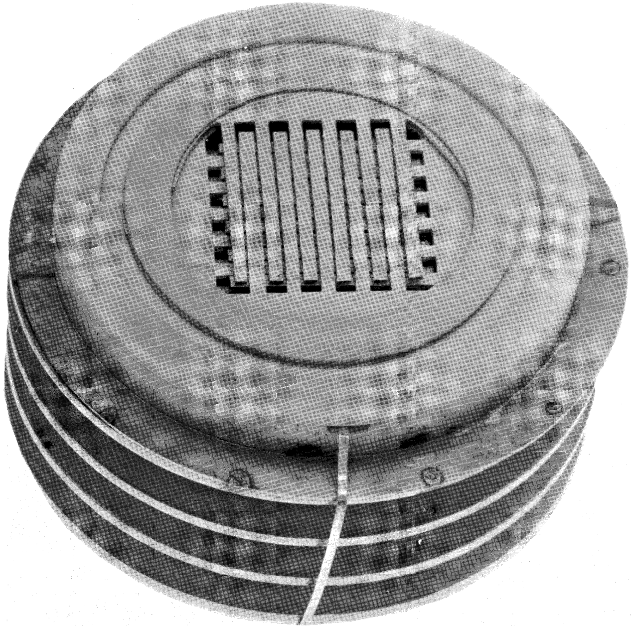
Figure 2. Completed assembly of 10 by 10 matrix fly's eye lens.
