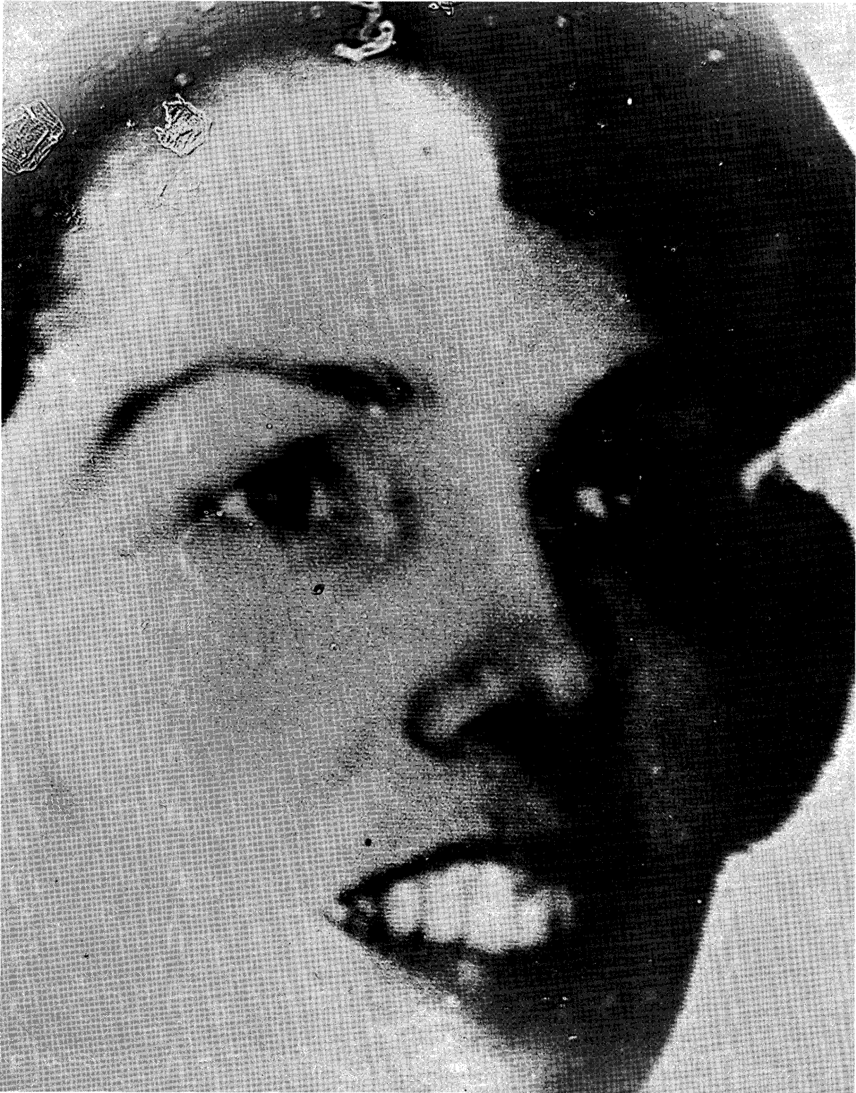
Figure 10. Portion of live image recording on photographic film. Scanning beam less than 1 micron on 2-micron centers.
