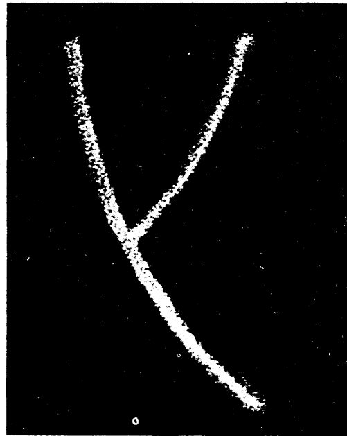
Figure 6—The real image of an optical reconstruction of the lambda in Figure 2
